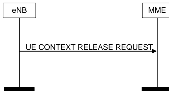
Figure 8.3.2.2-1: UE Context Release Request procedure. Successful operation.
