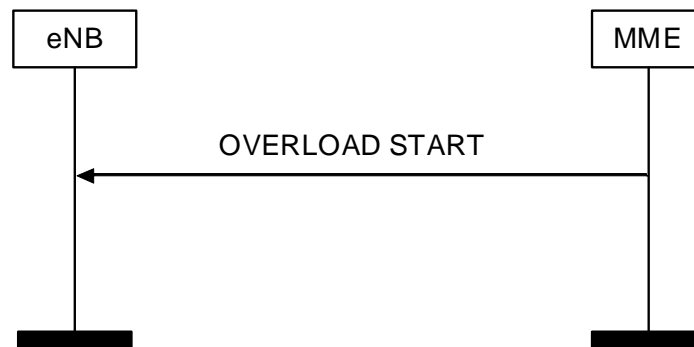
Figure 8.7.6.2-1: Overload Start procedure
