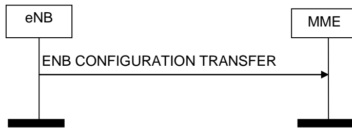
Figure 8.15.2.1-1: eNB Configuration Transfer procedure. Successful operation.
