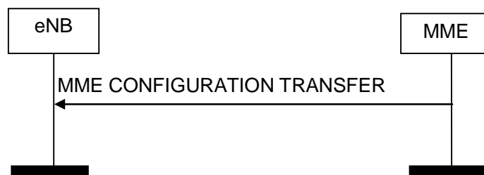
Figure 8.16.2.1-1: MME Configuration Transfer procedure. Successful operation.
