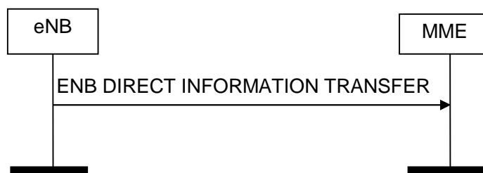
Figure 8.13.1.2-1: ENB Direct Information Transfer procedure. Successful operation.
