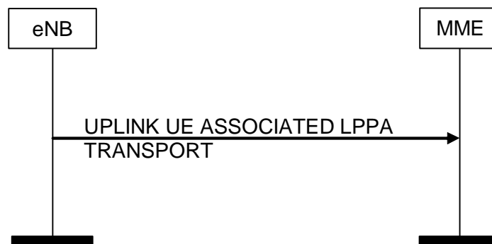
Figure 8.17.2.2-1: UPLINK UE ASSOCIATED LPPA TRANSPORT Procedure
