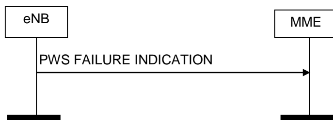
Figure 8.12.4.2-1: PWS Failure Indication procedure. Successful operation.
