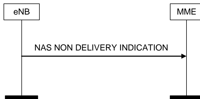
Figure 8.6.2.4-1: NAS NON DELIVERY INDICATION Procedure
