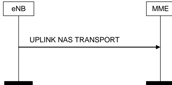
Figure 8.6.2.3-1: UPLINK NAS TRANSPORT Procedure
