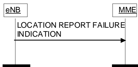
Figure 8.11.2.2-1: Location Report Failure Indication procedure.
