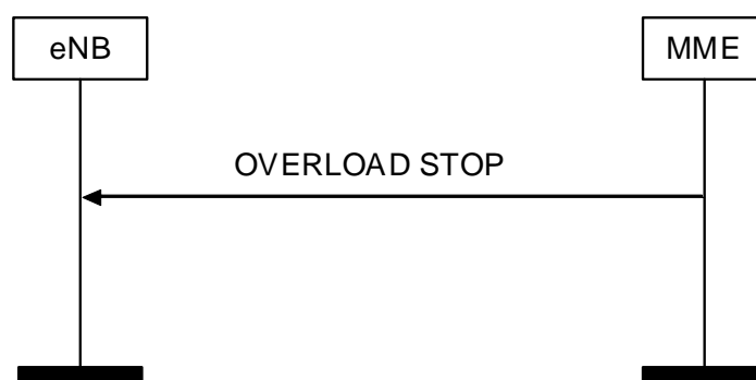
Figure 8.7.7.2.-1: Overload Stop procedure
