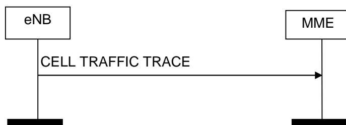
Figure 8.10.4.2-1: Cell Traffic Trace procedure. Successful operation.
