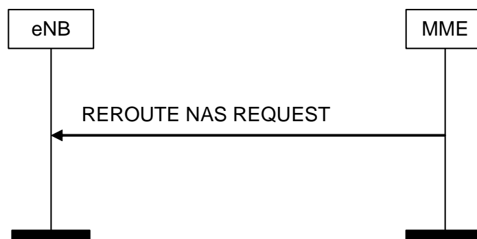
Figure 8.6.2.5-1: Reroute NAS Request Procedure
