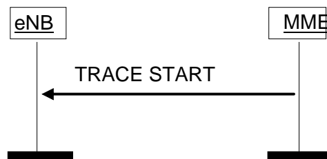
Figure 8.10.1.2-1: Trace Start procedure.
