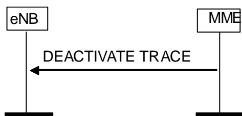
Figure 8.10.3.2-1: Deactivate Trace procedure. Successful operation.
