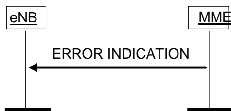
Figure 8.7.2.2-1: Error Indication procedure, MME originated. Successful operation.
