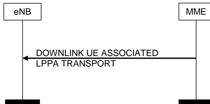
Figure 8.17.2.1-1: DOWNLINK UE ASSOCIATED LPPA Transport Procedure
