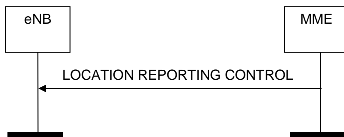
Figure 8.11.1.2-1: Location Reporting Control procedure. Successful operation.
