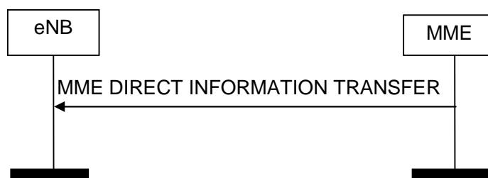
Figure 8.14.1.2-1: MME Direct Information Transfer procedure. Successful operation.
