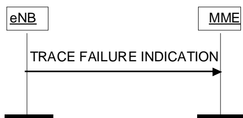
Figure 8.10.2.2-1: Trace Failure Indication procedure.
