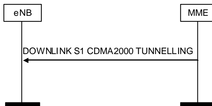
Figure 8.8.2.1-1: Downlink S1 CDMA2000 Tunnelling Procedure
