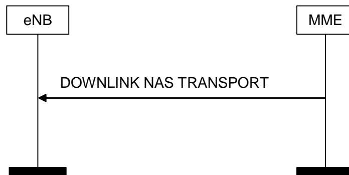
Figure 8.6.2.2-1: DOWNLINK NAS Transport Procedure
