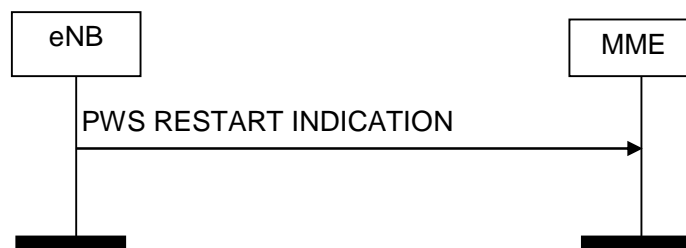
Figure 8.12.3.2-1: PWS Restart Indication procedure. Successful operation.
