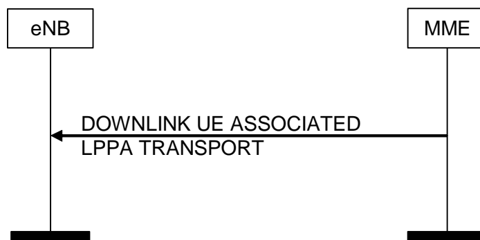
Figure 8.17.2.1-1: DOWNLINK UE ASSOCIATED LPPA Transport Procedure
