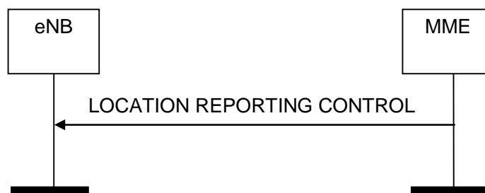
Figure 8.11.1.2-1: Location Reporting Control procedure. Successful operation.
