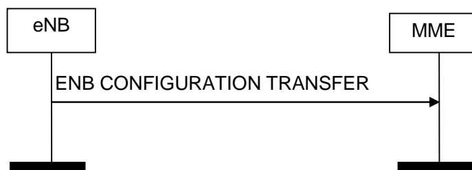
Figure 8.15.2.1-1: eNB Configuration Transfer procedure. Successful operation.
