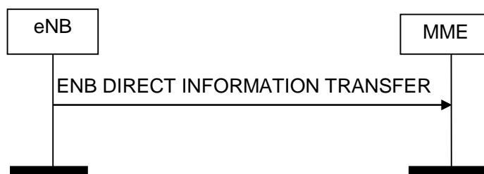
Figure 8.13.1.2-1: ENB Direct Information Transfer procedure. Successful operation.
