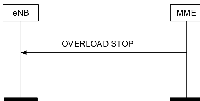
Figure 8.7.7.2.-1: Overload Stop procedure
