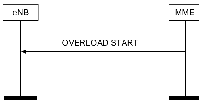
Figure 8.7.6.2-1: Overload Start procedure
