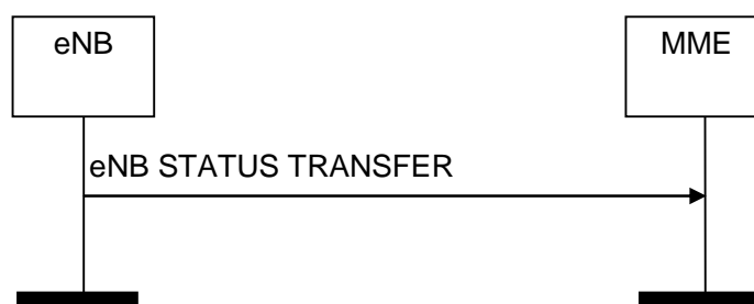
Figure 8.4.6.2-1: eNB Status Transfer procedure
