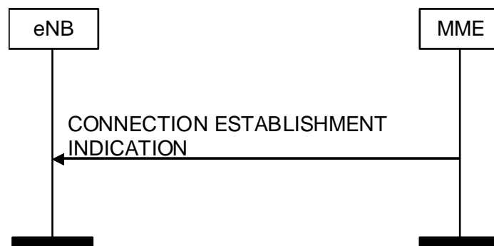
Figure 8.3.9.2-1: Connection Establishment Indication procedure. Successful operation.
