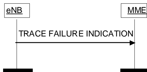
Figure 8.10.2.2-1: Trace Failure Indication procedure.
