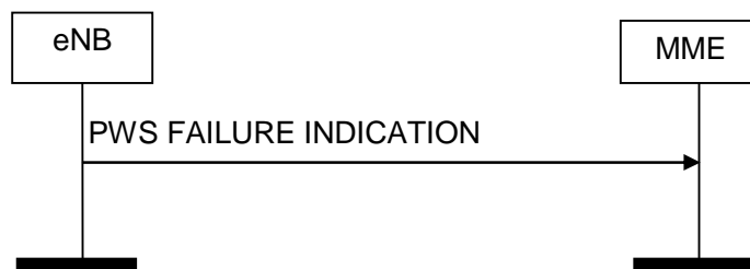
Figure 8.12.4.2-1: PWS Failure Indication procedure. Successful operation.
