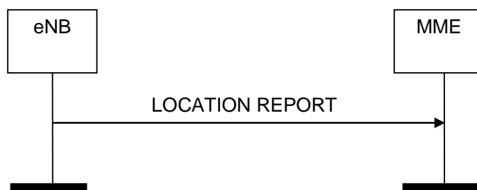
Figure 8.11.3.2-1: Location Report procedure. Successful operation.
