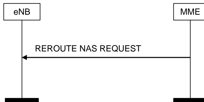
Figure 8.6.2.5-1: Reroute NAS Request Procedure
