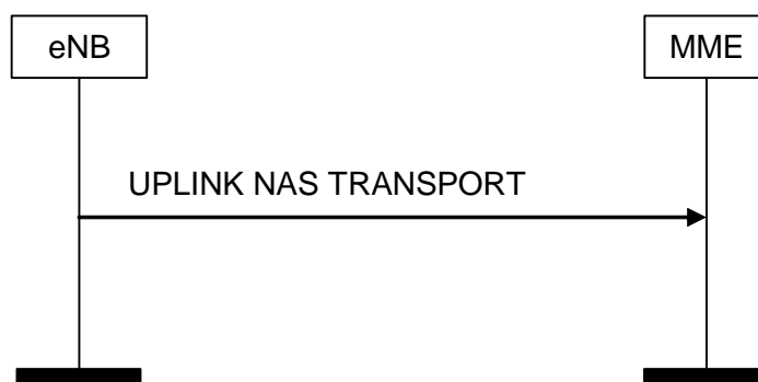
Figure 8.6.2.3-1: UPLINK NAS TRANSPORT Procedure
