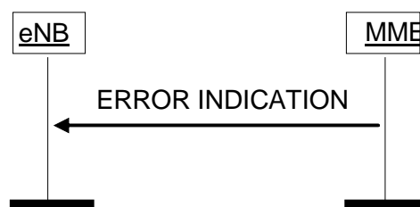
Figure 8.7.2.2-1: Error Indication procedure, MME originated. Successful operation.
