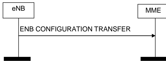
Figure 8.15.2.1-1: eNB Configuration Transfer procedure. Successful operation.
