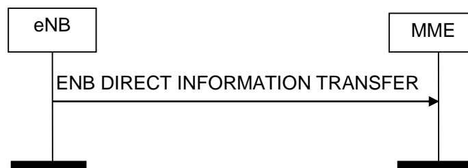
Figure 8.13.1.2-1: ENB Direct Information Transfer procedure. Successful operation.
