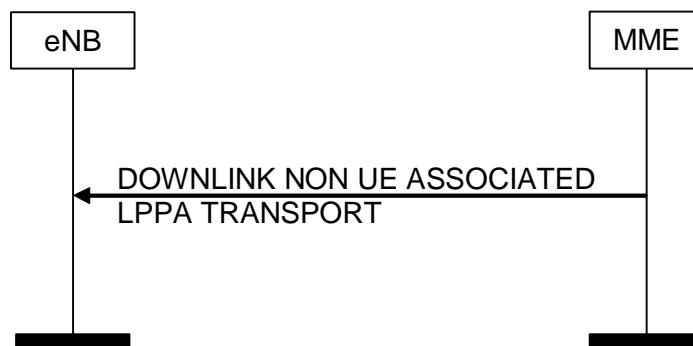
Figure 8.17.2.3-1: DOWNLINK NON UE ASSOCIATED LPPA Transport Procedure
