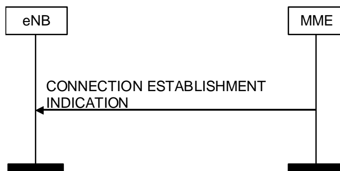
Figure 8.3.9.2-1: Connection Establishment Indication procedure. Successful operation.
