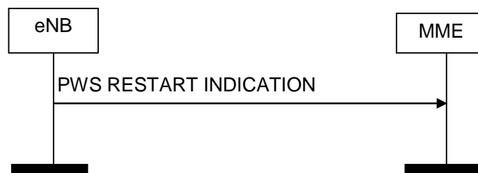
Figure 8.12.3.2-1: PWS Restart Indication procedure. Successful operation.
