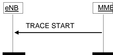
Figure 8.10.1.2-1: Trace Start procedure.
