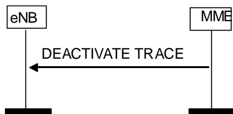
Figure 8.10.3.2-1: Deactivate Trace procedure. Successful operation.
