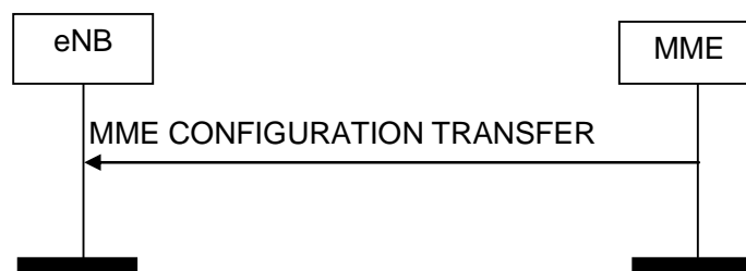
Figure 8.16.2.1-1: MME Configuration Transfer procedure. Successful operation.
