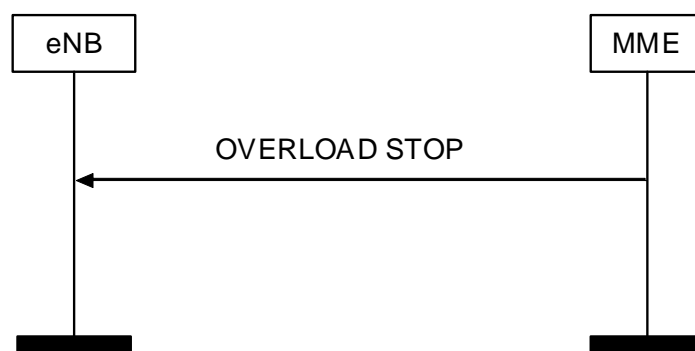
Figure 8.7.7.2.-1: Overload Stop procedure
