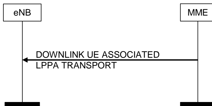
Figure 8.17.2.1-1: DOWNLINK UE ASSOCIATED LPPA Transport Procedure
