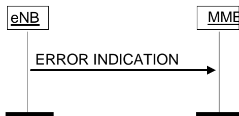
Figure 8.7.2.2-2: Error Indication procedure, eNB originated. Successful operation.
