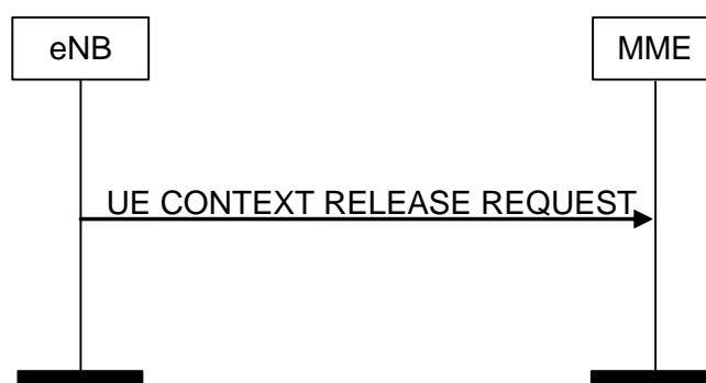
Figure 8.3.2.2-1: UE Context Release Request procedure. Successful operation.
