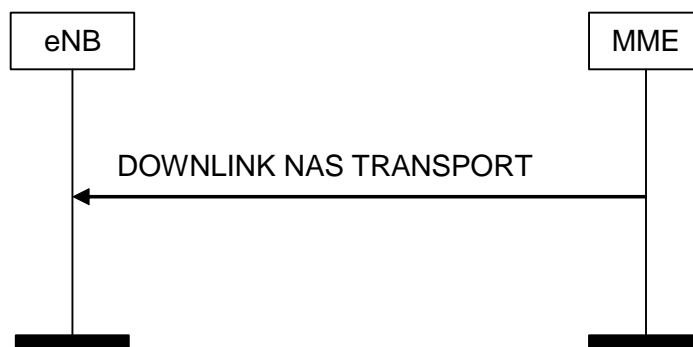
Figure 8.6.2.2-1: DOWNLINK NAS Transport Procedure
