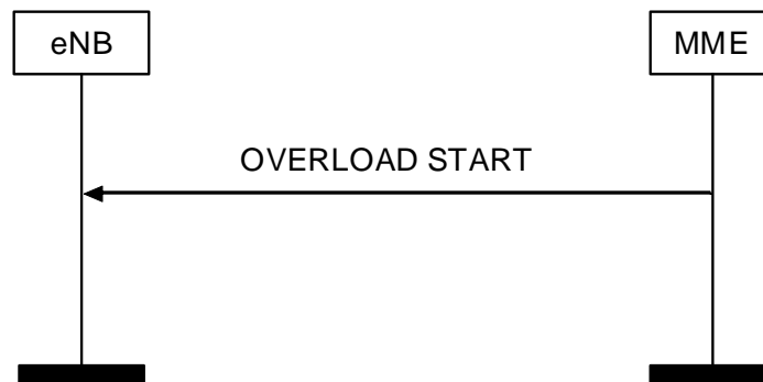
Figure 8.7.6.2-1: Overload Start procedure
