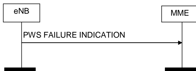
Figure 8.12.4.2-1: PWS Failure Indication procedure. Successful operation.
