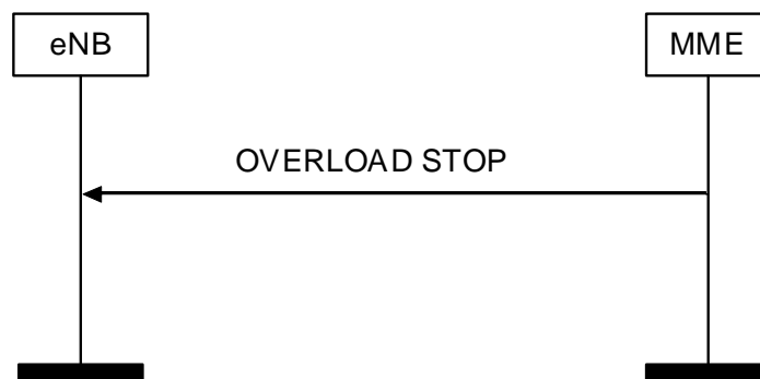
Figure 8.7.7.2.-1: Overload Stop procedure
