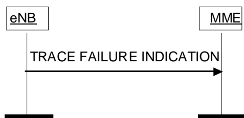
Figure 8.10.2.2-1: Trace Failure Indication procedure.
