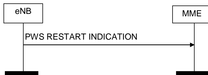
Figure 8.12.3.2-1: PWS Restart Indication procedure. Successful operation.
