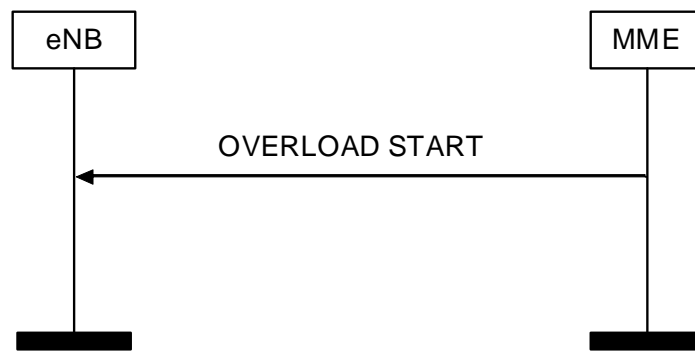
Figure 8.7.6.2-1: Overload Start procedure
