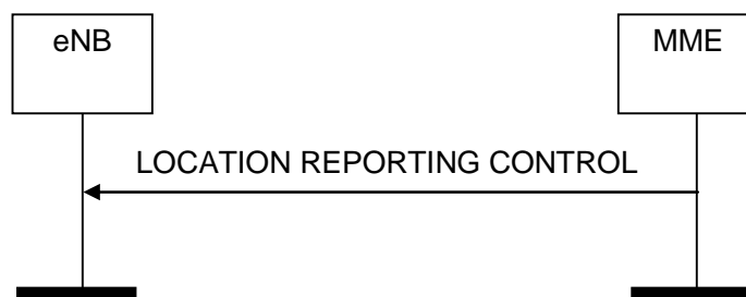
Figure 8.11.1.2-1: Location Reporting Control procedure. Successful operation.
