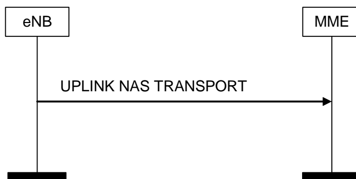
Figure 8.6.2.3-1: UPLINK NAS TRANSPORT Procedure
