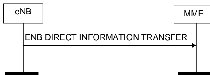
Figure 8.13.1.2-1: ENB Direct Information Transfer procedure. Successful operation.
