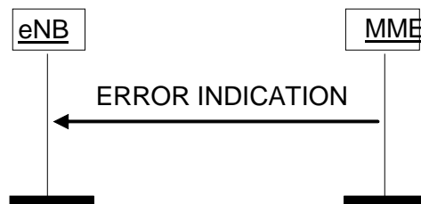
Figure 8.7.2.2-1: Error Indication procedure, MME originated. Successful operation.
