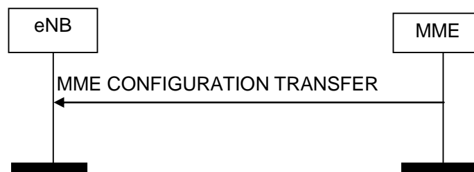
Figure 8.16.2.1-1: MME Configuration Transfer procedure. Successful operation.
