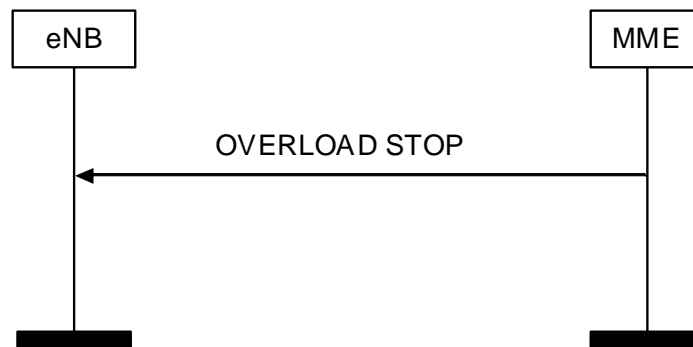
Figure 8.7.7.2.-1: Overload Stop procedure
