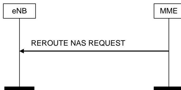
Figure 8.6.2.5-1: Reroute NAS Request Procedure
