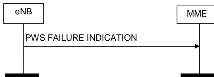
Figure 8.12.4.2-1: PWS Failure Indication procedure. Successful operation.
