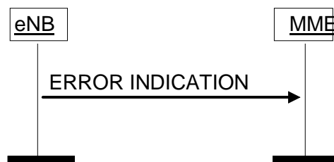
Figure 8.7.2.2-2: Error Indication procedure, eNB originated. Successful operation.
