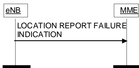
Figure 8.11.2.2-1: Location Report Failure Indication procedure.
