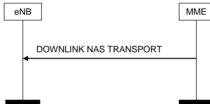
Figure 8.6.2.2-1: DOWNLINK NAS Transport Procedure
