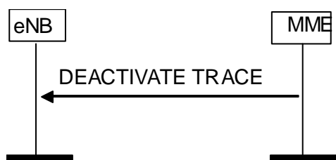
Figure 8.10.3.2-1: Deactivate Trace procedure. Successful operation.
