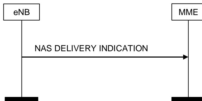
Figure 8.6.2.4a-1: NAS DELIVERY INDICATION Procedure
