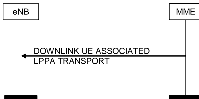
Figure 8.17.2.1-1: DOWNLINK UE ASSOCIATED LPPA Transport Procedure
