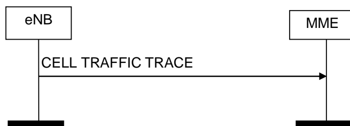
Figure 8.10.4.2-1: Cell Traffic Trace procedure. Successful operation.
