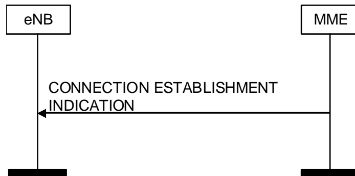
Figure 8.3.9.2-1: Connection Establishment Indication procedure. Successful operation.
