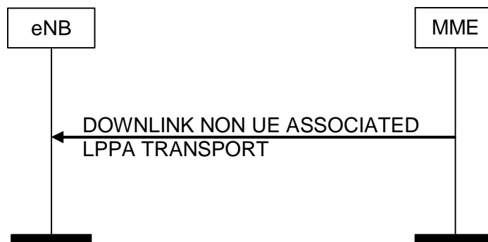
Figure 8.17.2.3-1: DOWNLINK NON UE ASSOCIATED LPPA Transport Procedure
