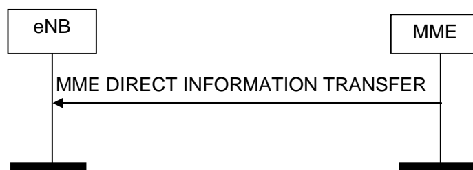
Figure 8.14.1.2-1: MME Direct Information Transfer procedure. Successful operation.
