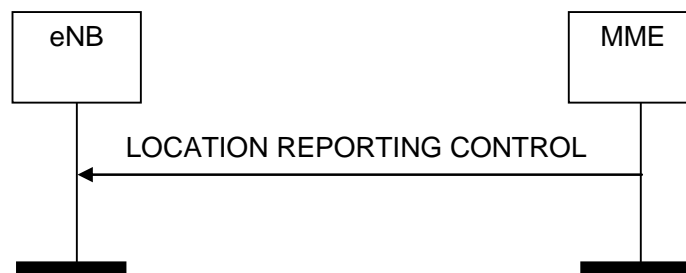
Figure 8.11.1.2-1: Location Reporting Control procedure. Successful operation.
