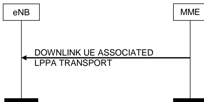
Figure 8.17.2.1-1: DOWNLINK UE ASSOCIATED LPPA Transport Procedure
