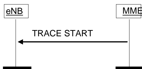
Figure 8.10.1.2-1: Trace Start procedure.
