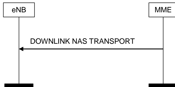
Figure 8.6.2.2-1: DOWNLINK NAS Transport Procedure
