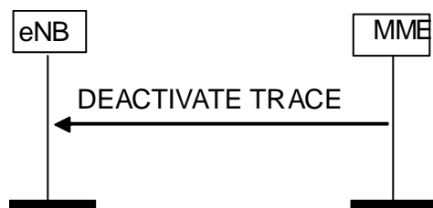
Figure 8.10.3.2-1: Deactivate Trace procedure. Successful operation.
