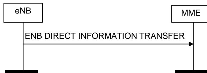
Figure 8.13.1.2-1: ENB Direct Information Transfer procedure. Successful operation.
