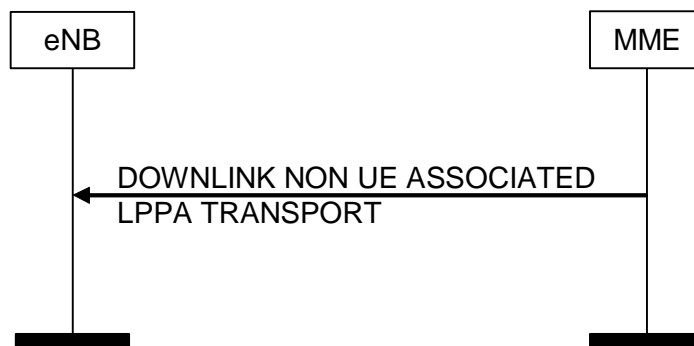
Figure 8.17.2.3-1: DOWNLINK NON UE ASSOCIATED LPPA Transport Procedure
