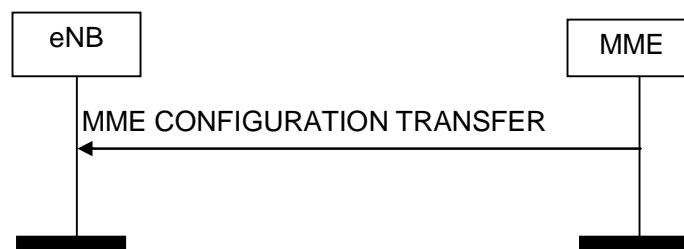
Figure 8.16.2.1-1: MME Configuration Transfer procedure. Successful operation.
