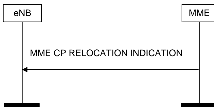
Figure 8.3.13.2-1: MME CP Relocation Indication. Successful operation.
