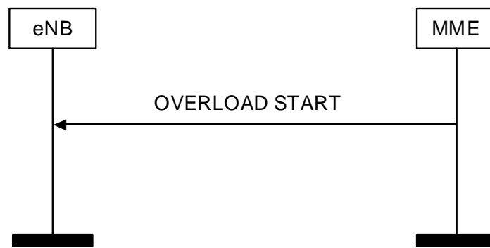
Figure 8.7.6.2-1: Overload Start procedure
