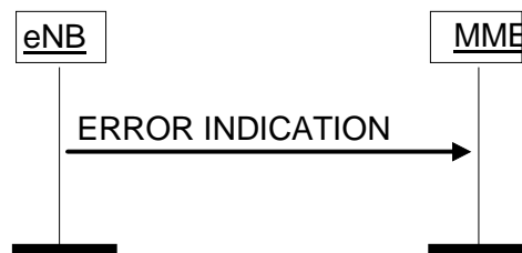
Figure 8.7.2.2-2: Error Indication procedure, eNB originated. Successful operation.
