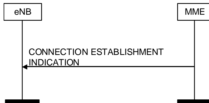
Figure 8.3.9.2-1: Connection Establishment Indication procedure. Successful operation.
