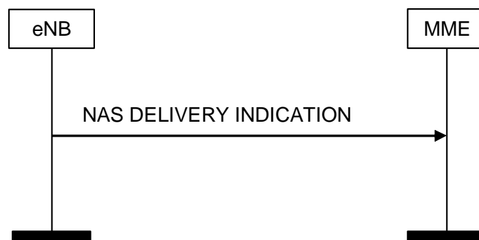
Figure 8.6.2.4a-1: NAS DELIVERY INDICATION Procedure
