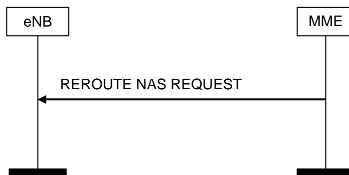
Figure 8.6.2.5-1: Reroute NAS Request Procedure
