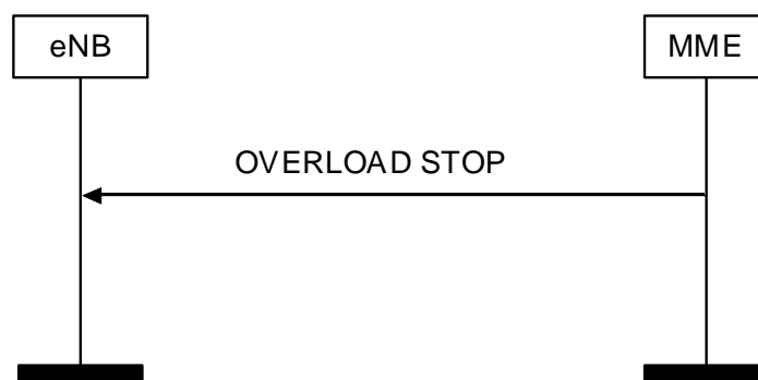
Figure 8.7.7.2.-1: Overload Stop procedure
