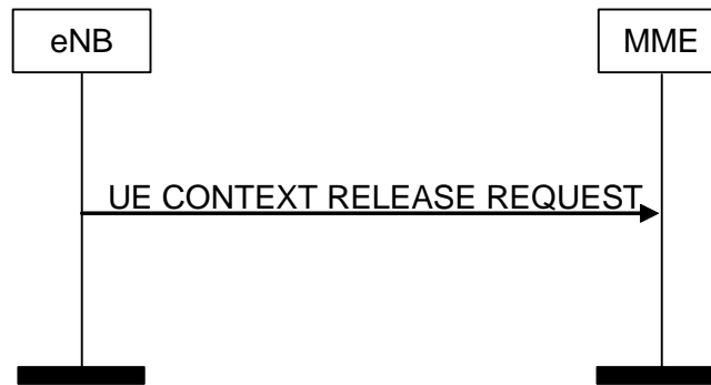
Figure 8.3.2.2-1: UE Context Release Request procedure. Successful operation.
