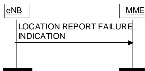
Figure 8.11.2.2-1: Location Report Failure Indication procedure.
