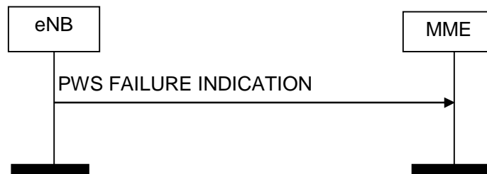
Figure 8.12.4.2-1: PWS Failure Indication procedure. Successful operation.
