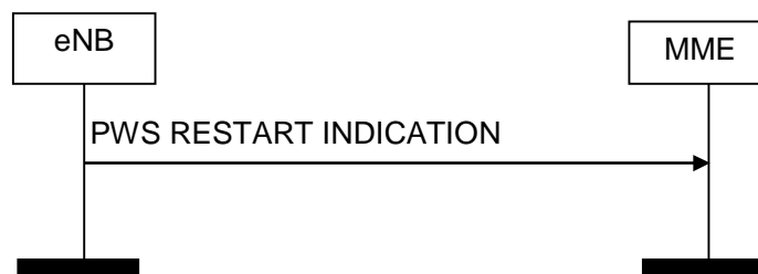
Figure 8.12.3.2-1: PWS Restart Indication procedure. Successful operation.
