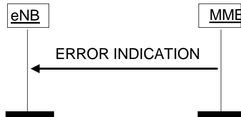
Figure 8.7.2.2-1: Error Indication procedure, MME originated. Successful operation.
