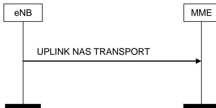
Figure 8.6.2.3-1: UPLINK NAS TRANSPORT Procedure
