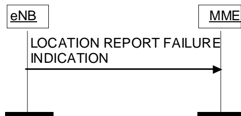
Figure 8.11.2.2-1: Location Report Failure Indication procedure.
