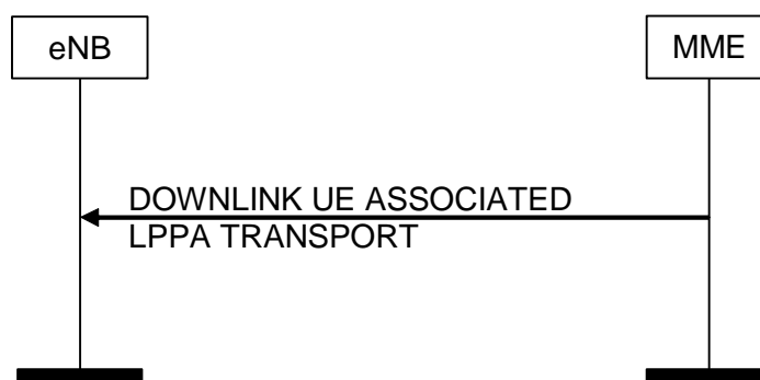
Figure 8.17.2.1-1: DOWNLINK UE ASSOCIATED LPPA Transport Procedure
