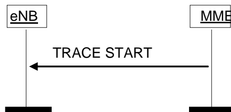
Figure 8.10.1.2-1: Trace Start procedure.
