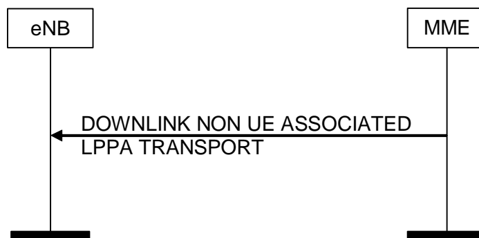
Figure 8.17.2.3-1: DOWNLINK NON UE ASSOCIATED LPPA Transport Procedure
