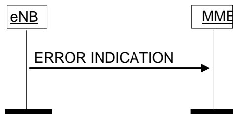
Figure 8.7.2.2-2: Error Indication procedure, eNB originated. Successful operation.
