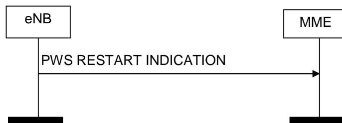
Figure 8.12.3.2-1: PWS Restart Indication procedure. Successful operation.
