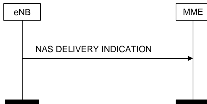
Figure 8.6.2.4a-1: NAS DELIVERY INDICATION Procedure
