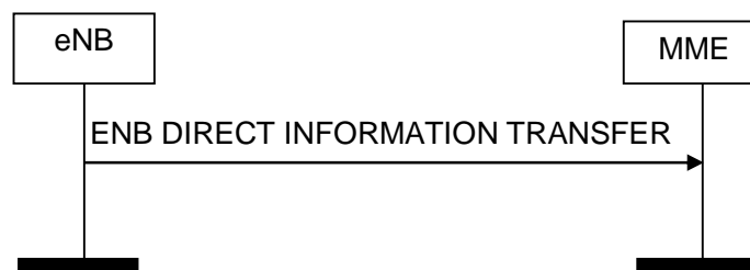
Figure 8.13.1.2-1: ENB Direct Information Transfer procedure. Successful operation.
