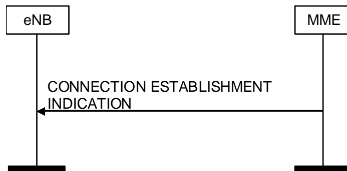
Figure 8.3.9.2-1: Connection Establishment Indication procedure. Successful operation.
