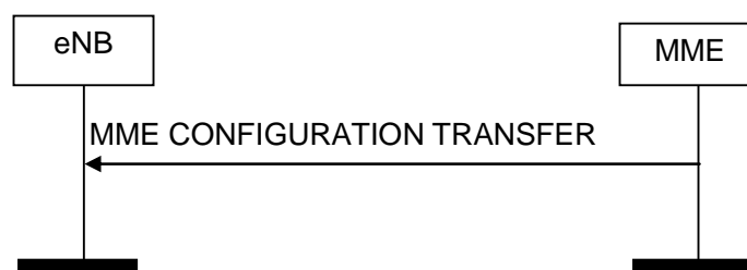
Figure 8.16.2.1-1: MME Configuration Transfer procedure. Successful operation.
