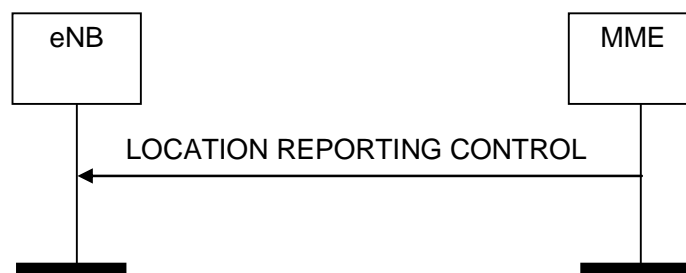
Figure 8.11.1.2-1: Location Reporting Control procedure. Successful operation.
