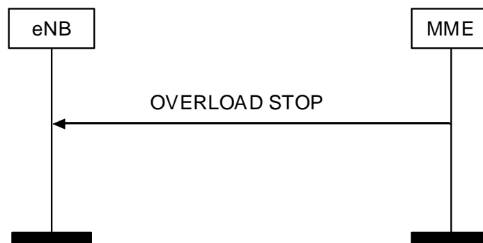
Figure 8.7.7.2.-1: Overload Stop procedure
