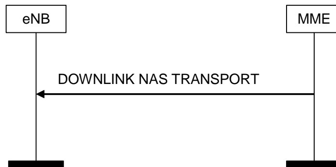
Figure 8.6.2.2-1: DOWNLINK NAS Transport Procedure
