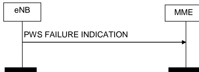
Figure 8.12.4.2-1: PWS Failure Indication procedure. Successful operation.
