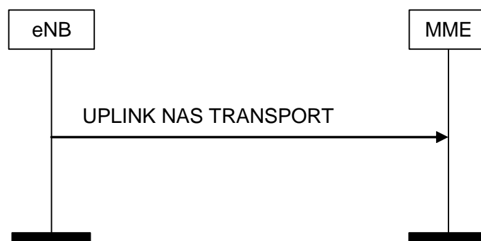
Figure 8.6.2.3-1: UPLINK NAS TRANSPORT Procedure
