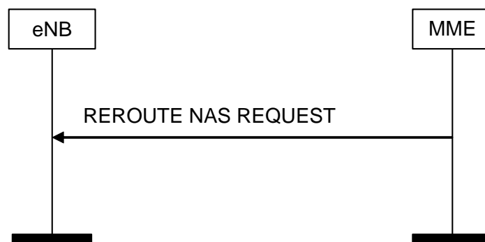
Figure 8.6.2.5-1: Reroute NAS Request Procedure
