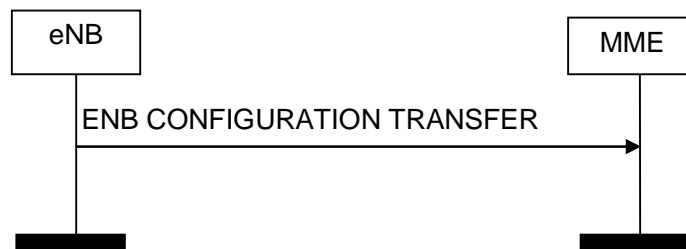
Figure 8.15.2.1-1: eNB Configuration Transfer procedure. Successful operation.
