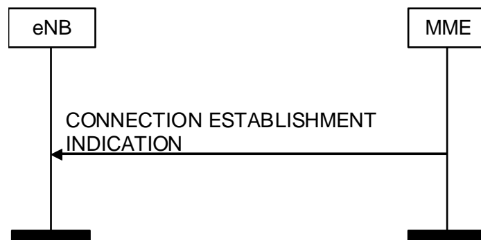
Figure 8.3.9.2-1: Connection Establishment Indication procedure. Successful operation.
