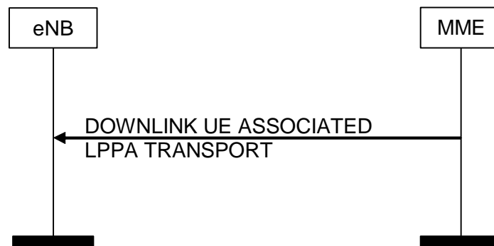
Figure 8.17.2.1-1: DOWNLINK UE ASSOCIATED LPPA Transport Procedure
