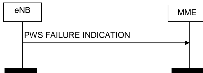
Figure 8.12.4.2-1: PWS Failure Indication procedure. Successful operation.
