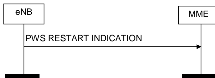
Figure 8.12.3.2-1: PWS Restart Indication procedure. Successful operation.
