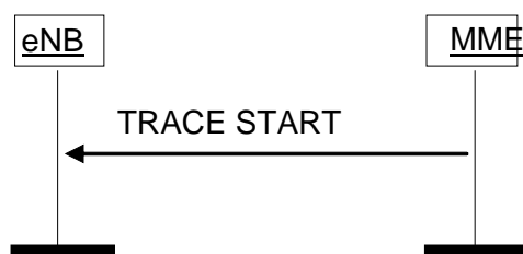
Figure 8.10.1.2-1: Trace Start procedure.
