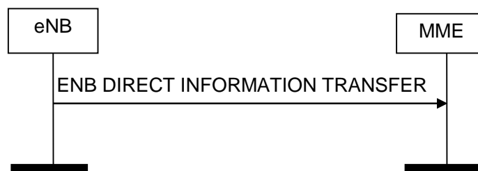
Figure 8.13.1.2-1: ENB Direct Information Transfer procedure. Successful operation.
