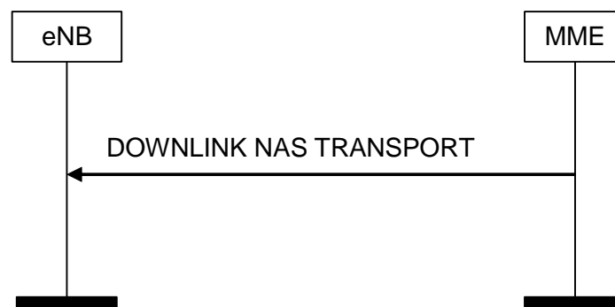
Figure 8.6.2.2-1: DOWNLINK NAS Transport Procedure
