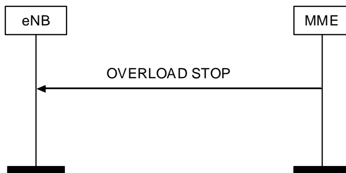
Figure 8.7.7.2.-1: Overload Stop procedure
