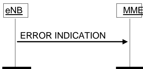
Figure 8.7.2.2-2: Error Indication procedure, eNB originated. Successful operation.
