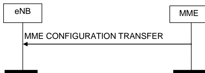
Figure 8.16.2.1-1: MME Configuration Transfer procedure. Successful operation.
