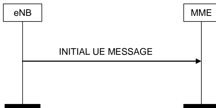
Figure 8.6.2.1-1: Initial UE Message procedure
