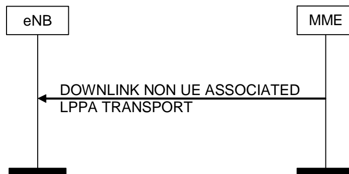
Figure 8.17.2.3-1: DOWNLINK NON UE ASSOCIATED LPPA Transport Procedure
