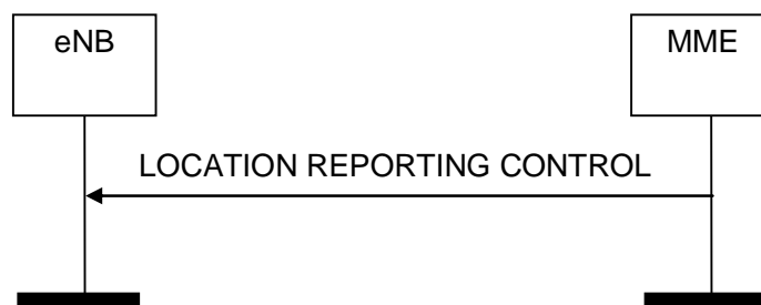
Figure 8.11.1.2-1: Location Reporting Control procedure. Successful operation.
