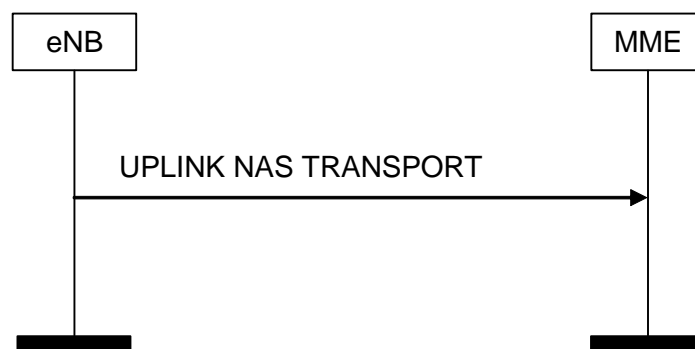
Figure 8.6.2.3-1: UPLINK NAS TRANSPORT Procedure
