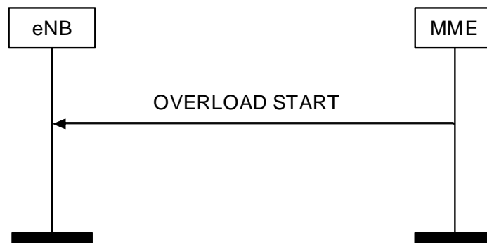
Figure 8.7.6.2-1: Overload Start procedure
