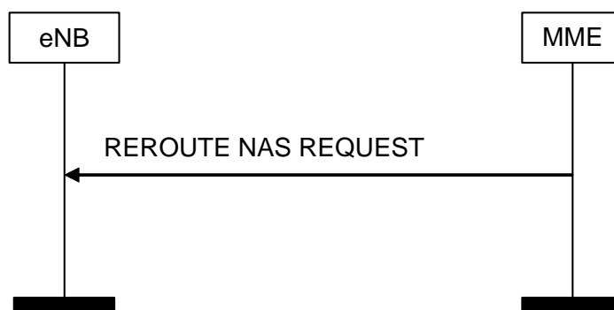
Figure 8.6.2.5-1: Reroute NAS Request Procedure
