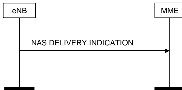
Figure 8.6.2.4a-1: NAS DELIVERY INDICATION Procedure
