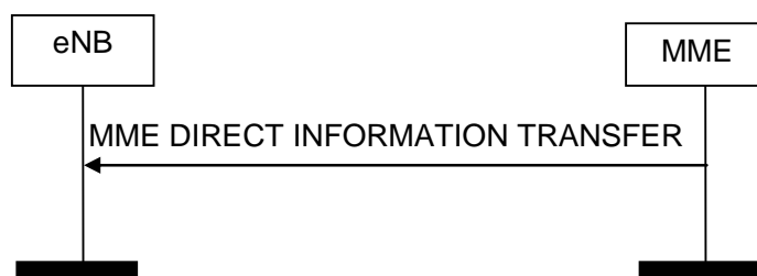
Figure 8.14.1.2-1: MME Direct Information Transfer procedure. Successful operation.
