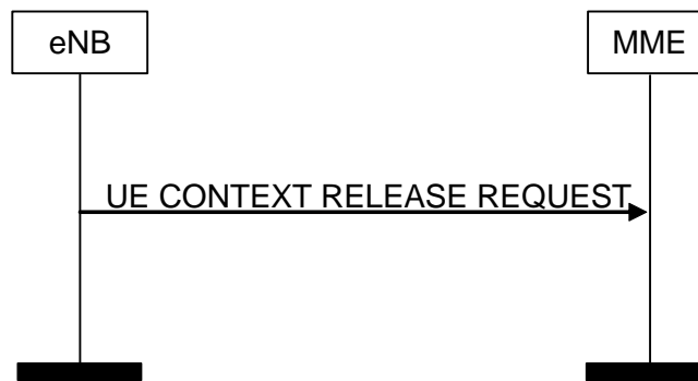
Figure 8.3.2.2-1: UE Context Release Request procedure. Successful operation.
