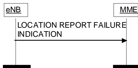
Figure 8.11.2.2-1: Location Report Failure Indication procedure.
