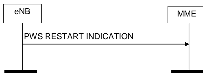
Figure 8.12.3.2-1: PWS Restart Indication procedure. Successful operation.
