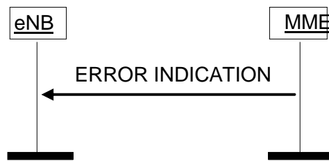
Figure 8.7.2.2-1: Error Indication procedure, MME originated. Successful operation.
