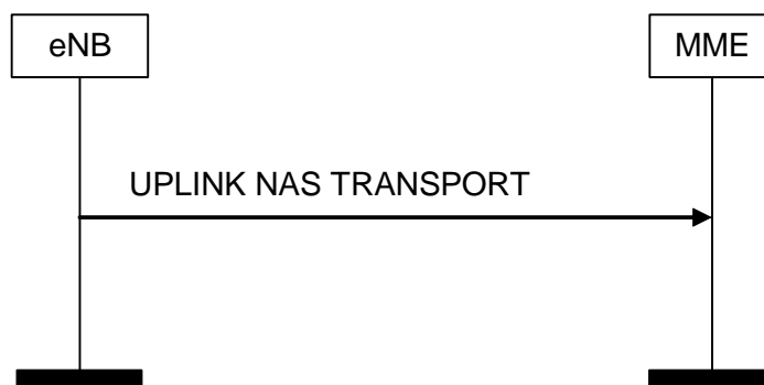
Figure 8.6.2.3-1: UPLINK NAS TRANSPORT Procedure
