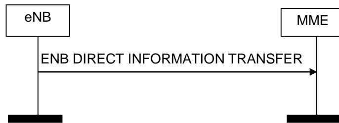
Figure 8.13.1.2-1: ENB Direct Information Transfer procedure. Successful operation.
