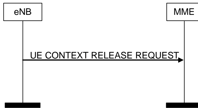
Figure 8.3.2.2-1: UE Context Release Request procedure. Successful operation.
