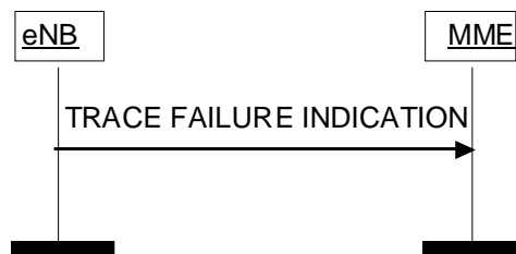
Figure 8.10.2.2-1: Trace Failure Indication procedure.
