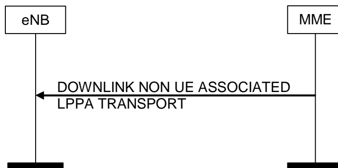
Figure 8.17.2.3-1: DOWNLINK NON UE ASSOCIATED LPPA Transport Procedure
