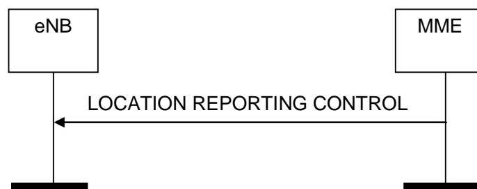
Figure 8.11.1.2-1: Location Reporting Control procedure. Successful operation.
