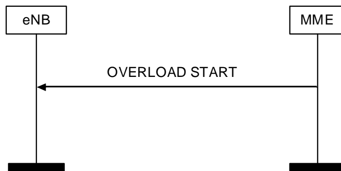
Figure 8.7.6.2-1: Overload Start procedure
