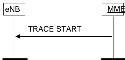
Figure 8.10.1.2-1: Trace Start procedure.
