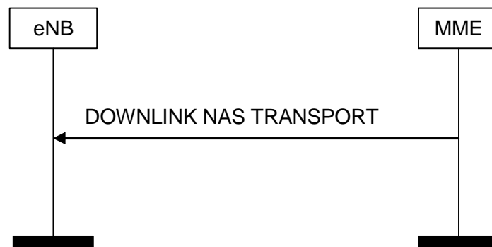
Figure 8.6.2.2-1: DOWNLINK NAS Transport Procedure
