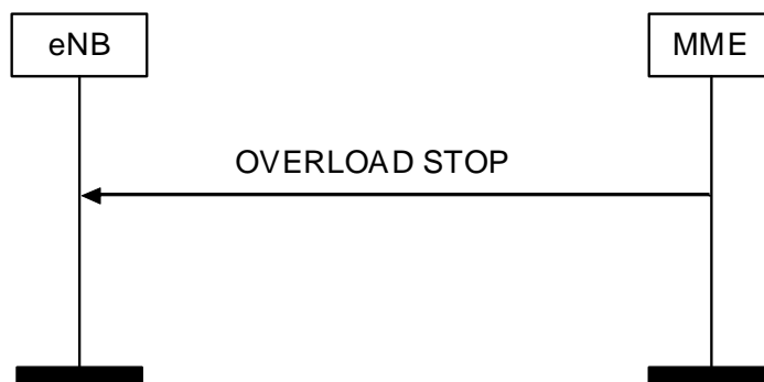
Figure 8.7.7.2.-1: Overload Stop procedure
