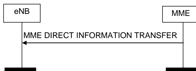
Figure 8.14.1.2-1: MME Direct Information Transfer procedure. Successful operation.
