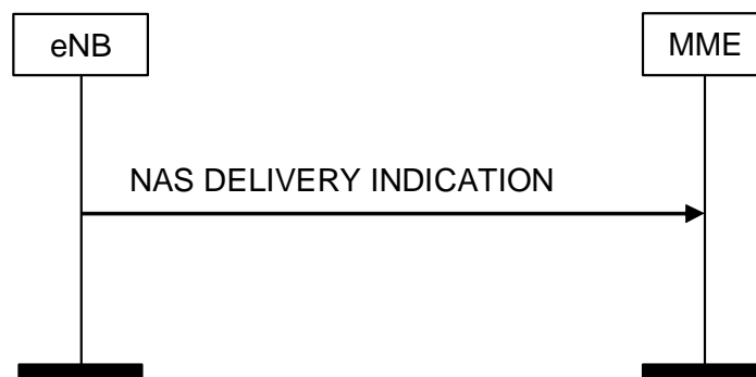
Figure 8.6.2.4a-1: NAS DELIVERY INDICATION Procedure
