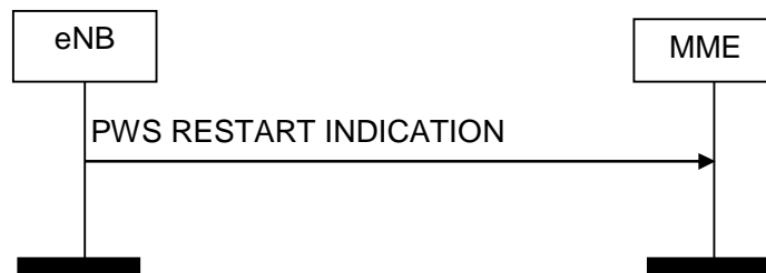
Figure 8.12.3.2-1: PWS Restart Indication procedure. Successful operation.
