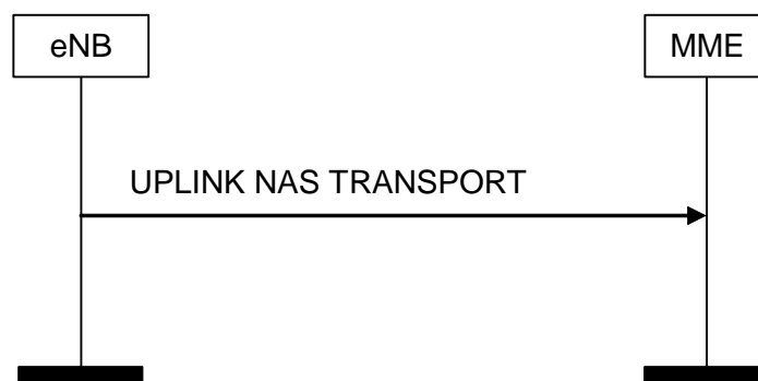
Figure 8.6.2.3-1: UPLINK NAS TRANSPORT Procedure
