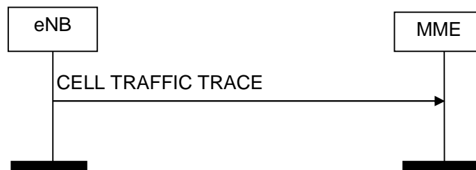
Figure 8.10.4.2-1: Cell Traffic Trace procedure. Successful operation.
