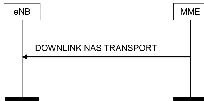
Figure 8.6.2.2-1: DOWNLINK NAS Transport Procedure
