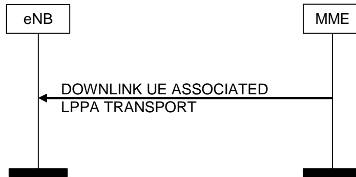
Figure 8.17.2.1-1: DOWNLINK UE ASSOCIATED LPPA Transport Procedure
