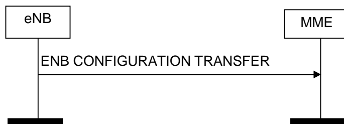
Figure 8.15.2.1-1: eNB Configuration Transfer procedure. Successful operation.
