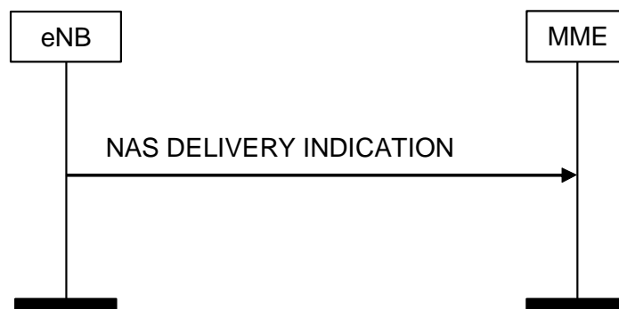
Figure 8.6.2.4a-1: NAS DELIVERY INDICATION Procedure
