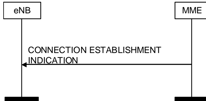
Figure 8.3.9.2-1: Connection Establishment Indication procedure. Successful operation.
