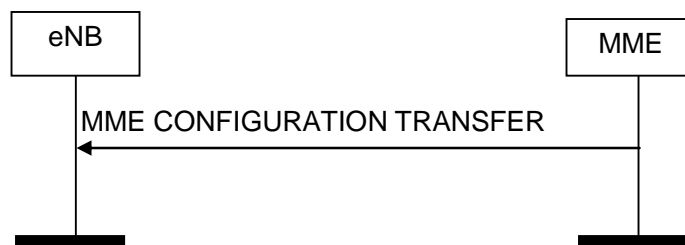
Figure 8.16.2.1-1: MME Configuration Transfer procedure. Successful operation.
