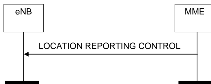
Figure 8.11.1.2-1: Location Reporting Control procedure. Successful operation.
