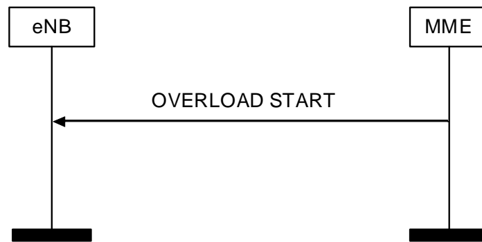
Figure 8.7.6.2-1: Overload Start procedure
