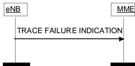
Figure 8.10.2.2-1: Trace Failure Indication procedure.
