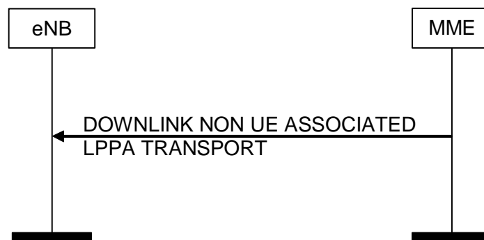
Figure 8.17.2.3-1: DOWNLINK NON UE ASSOCIATED LPPA Transport Procedure
