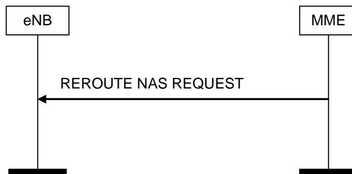
Figure 8.6.2.5-1: Reroute NAS Request Procedure
