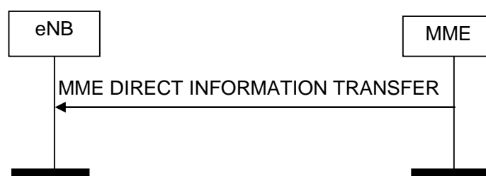
Figure 8.14.1.2-1: MME Direct Information Transfer procedure. Successful operation.
