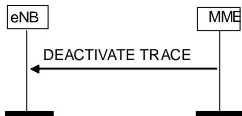
Figure 8.10.3.2-1: Deactivate Trace procedure. Successful operation.
