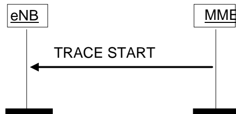
Figure 8.10.1.2-1: Trace Start procedure.
