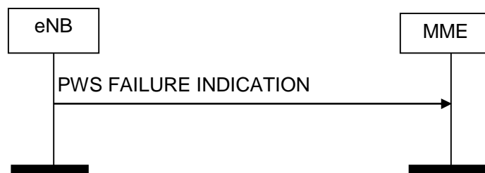
Figure 8.12.4.2-1: PWS Failure Indication procedure. Successful operation.
