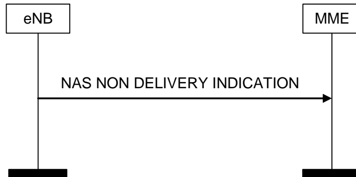
Figure 8.6.2.4-1: NAS NON DELIVERY INDICATION Procedure
