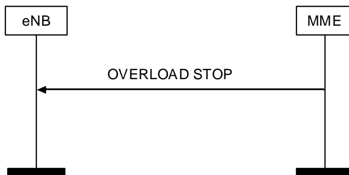
Figure 8.7.7.2.-1: Overload Stop procedure
