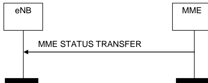
Figure 8.4.7.2-1: MME Status Transfer procedure
