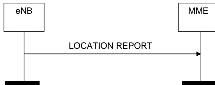
Figure 8.11.3.2-1: Location Report procedure. Successful operation.
