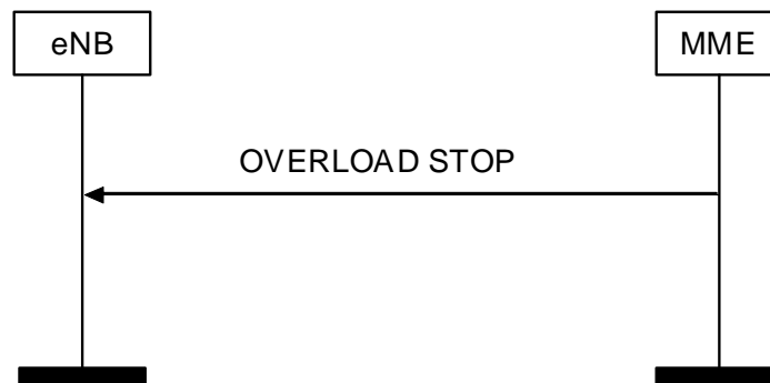
Figure 8.7.7.2.-1: Overload Stop procedure
