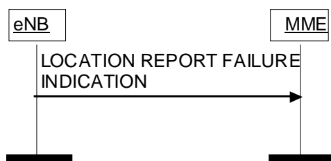
Figure 8.11.2.2-1: Location Report Failure Indication procedure.
