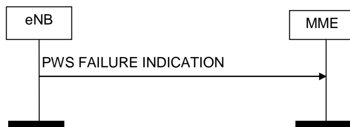
Figure 8.12.4.2-1: PWS Failure Indication procedure. Successful operation.
