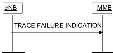
Figure 8.10.2.2-1: Trace Failure Indication procedure.
