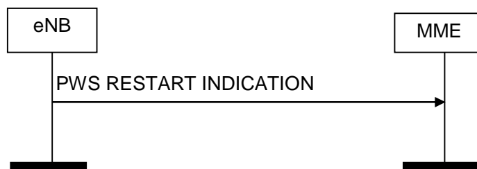
Figure 8.12.3.2-1: PWS Restart Indication procedure. Successful operation.
