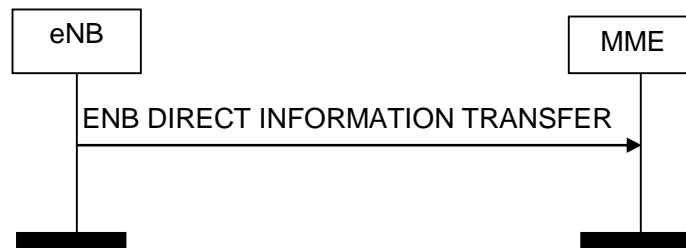
Figure 8.13.1.2-1: ENB Direct Information Transfer procedure. Successful operation.
