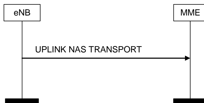
Figure 8.6.2.3-1: UPLINK NAS TRANSPORT Procedure
