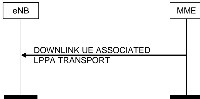
Figure 8.17.2.1-1: DOWNLINK UE ASSOCIATED LPPA Transport Procedure
