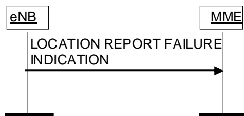
Figure 8.11.2.2-1: Location Report Failure Indication procedure.
