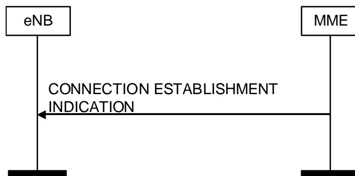
Figure 8.3.9.2-1: Connection Establishment Indication procedure. Successful operation.
