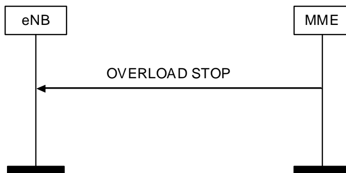
Figure 8.7.7.2.-1: Overload Stop procedure
