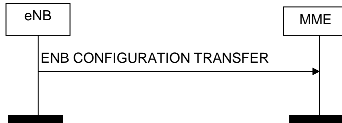
Figure 8.15.2.1-1: eNB Configuration Transfer procedure. Successful operation.
