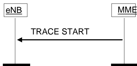
Figure 8.10.1.2-1: Trace Start procedure.
