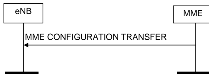
Figure 8.16.2.1-1: MME Configuration Transfer procedure. Successful operation.
