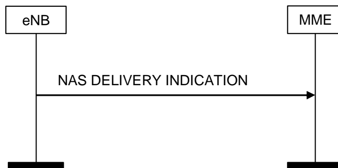
Figure 8.6.2.4a-1: NAS DELIVERY INDICATION Procedure
