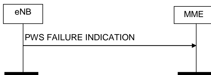
Figure 8.12.4.2-1: PWS Failure Indication procedure. Successful operation.
