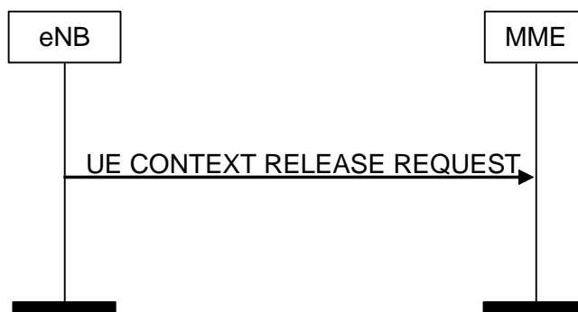
Figure 8.3.2-1: UE Context Release Request procedure. Successful operation.
