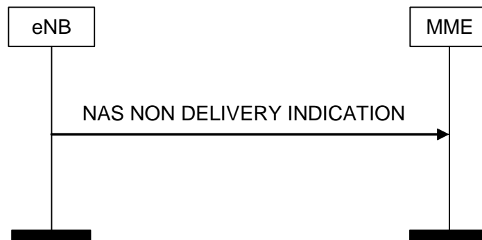
Figure 8.6.2.4-1: NAS NON DELIVERY INDICATION Procedure
