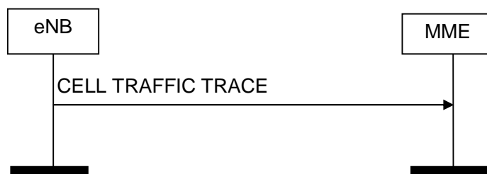
Figure 8.10.4.2-1: Cell Traffic Trace procedure. Successful operation.
