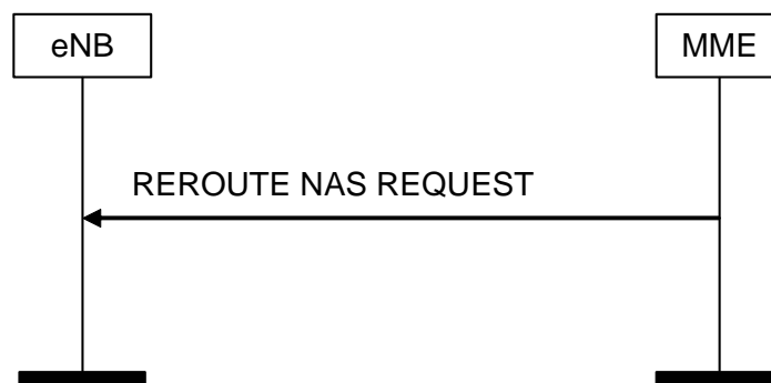
Figure 8.6.2.5-1: Reroute NAS Request Procedure
