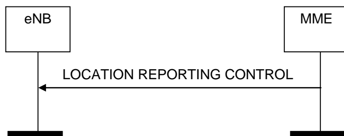
Figure 8.11.1.2-1: Location Reporting Control procedure. Successful operation.
