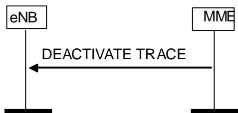
Figure 8.10.3.2-1: Deactivate Trace procedure. Successful operation.
