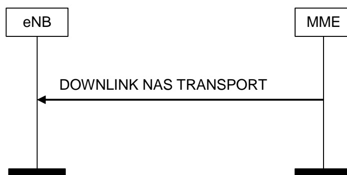
Figure 8.6.2.2-1: DOWNLINK NAS Transport Procedure
