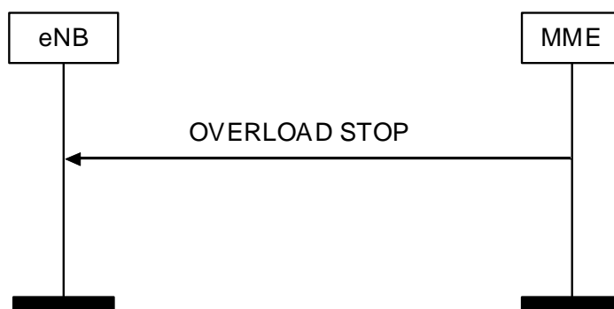
Figure 8.7.7.2.-1: Overload Stop procedure
