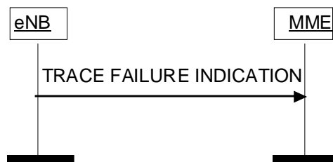
Figure 8.10.2.2-1: Trace Failure Indication procedure.
