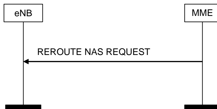
Figure 8.6.2.5-1: Reroute NAS Request Procedure
