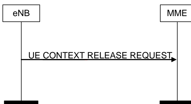
Figure 8.3.2.2-1: UE Context Release Request procedure. Successful operation.
