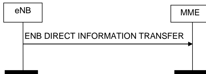
Figure 8.13.1.2-1: ENB Direct Information Transfer procedure. Successful operation.
