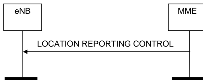
Figure 8.11.1.2-1: Location Reporting Control procedure. Successful operation.
