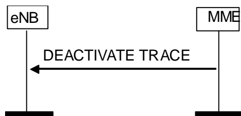
Figure 8.10.3.2-1: Deactivate Trace procedure. Successful operation.
