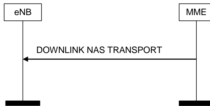
Figure 8.6.2.2-1: DOWNLINK NAS Transport Procedure
