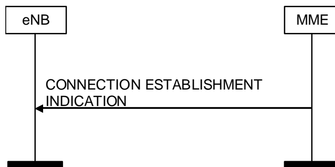
Figure 8.3.9.2-1: Connection Establishment Indication procedure. Successful operation.
