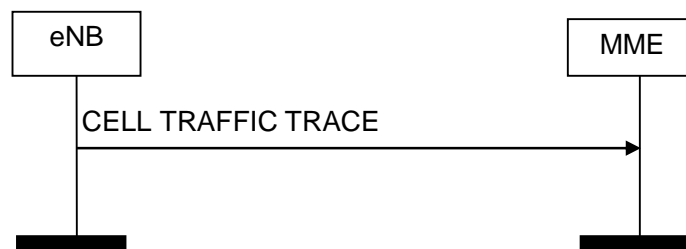
Figure 8.10.4.2-1: Cell Traffic Trace procedure. Successful operation.
