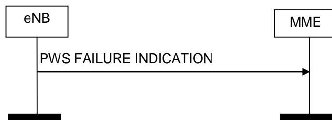
Figure 8.12.4.2-1: PWS Failure Indication procedure. Successful operation.
