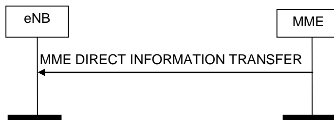
Figure 8.14.1.2-1: MME Direct Information Transfer procedure. Successful operation.
