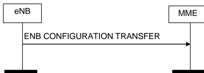
Figure 8.15.2.1-1: eNB Configuration Transfer procedure. Successful operation.
