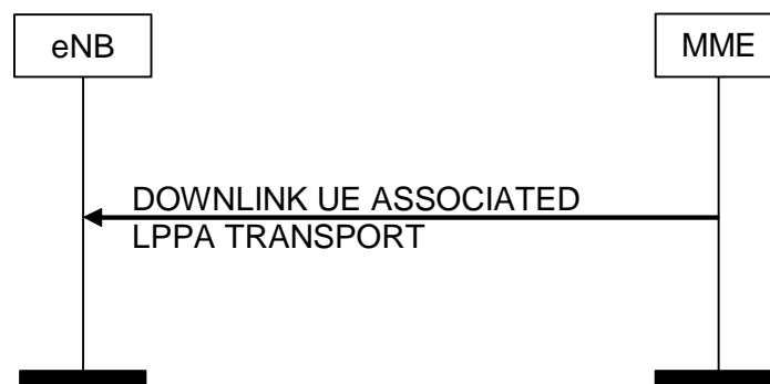
Figure 8.17.2.1-1: DOWNLINK UE ASSOCIATED LPPA Transport Procedure
