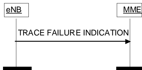
Figure 8.10.2.2-1: Trace Failure Indication procedure.
