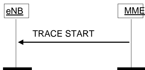
Figure 8.10.1.2-1: Trace Start procedure.
