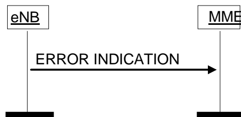
Figure 8.7.2.2-2: Error Indication procedure, eNB originated. Successful operation.
