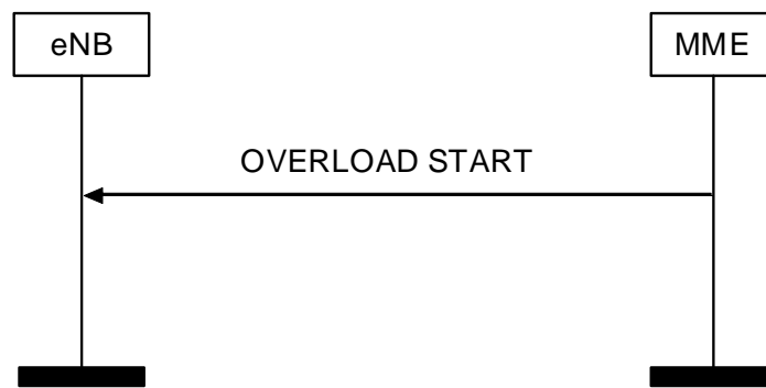
Figure 8.7.6.2-1: Overload Start procedure
