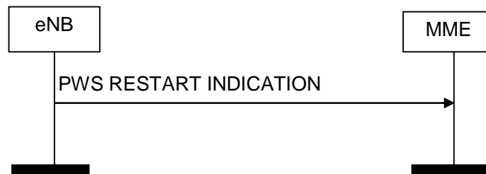
Figure 8.12.3.2-1: PWS Restart Indication procedure. Successful operation.
