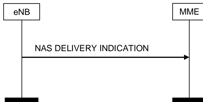
Figure 8.6.2.4a-1: NAS DELIVERY INDICATION Procedure
