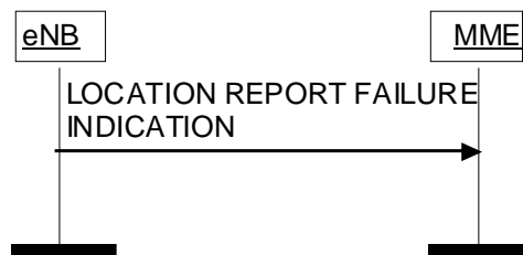
Figure 8.11.2.2-1: Location Report Failure Indication procedure.
