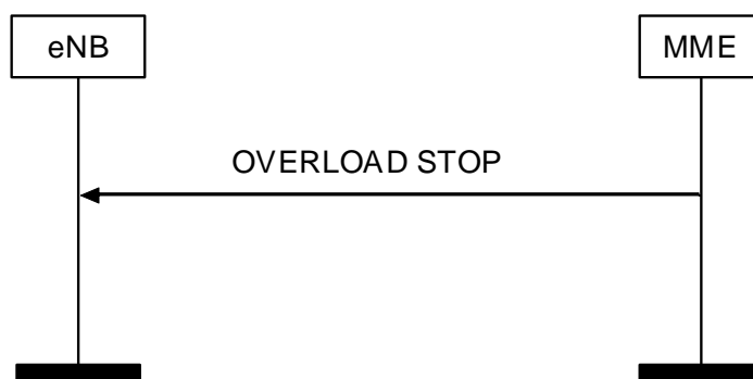
Figure 8.7.7.2.-1: Overload Stop procedure
