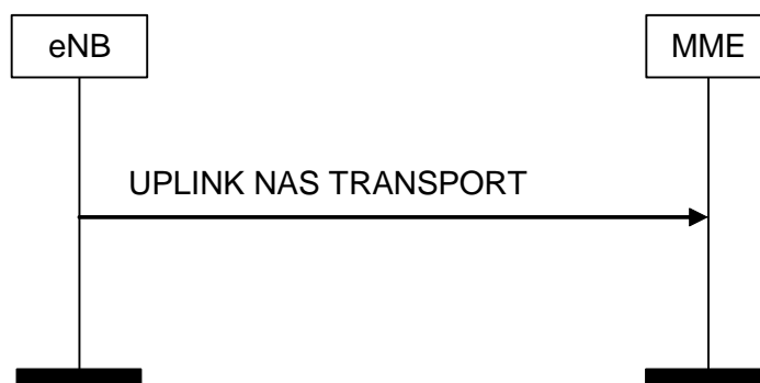
Figure 8.6.2.3-1: UPLINK NAS TRANSPORT Procedure
