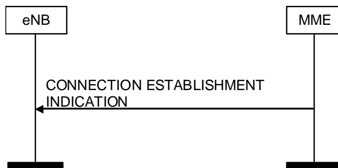
Figure 8.3.9.2-1: Connection Establishment Indication procedure. Successful operation.
