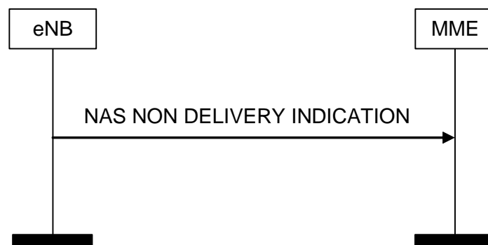
Figure 8.6.2.4-1: NAS NON DELIVERY INDICATION Procedure
