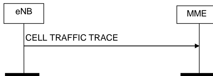
Figure 8.10.4.2-1: Cell Traffic Trace procedure. Successful operation.
