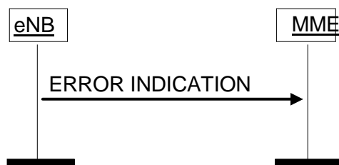
Figure 8.7.2.2-2: Error Indication procedure, eNB originated. Successful operation.
