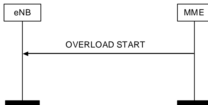
Figure 8.7.6.2-1: Overload Start procedure
