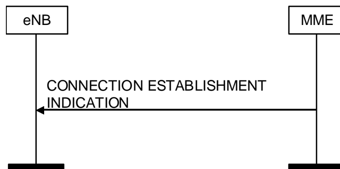
Figure 8.3.9.2-1: Connection Establishment Indication procedure. Successful operation.
