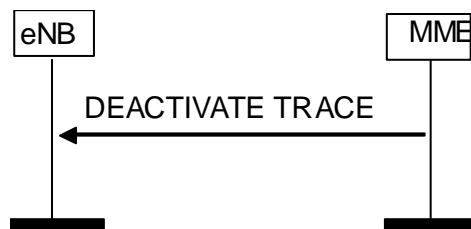
Figure 8.10.3.2-1: Deactivate Trace procedure. Successful operation.
