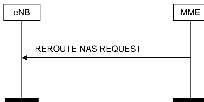
Figure 8.6.2.5-1: Reroute NAS Request Procedure
