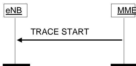
Figure 8.10.1.2-1: Trace Start procedure.
