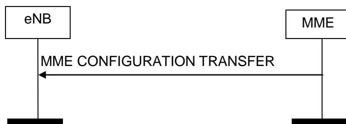
Figure 8.16.2.1-1: MME Configuration Transfer procedure. Successful operation.
