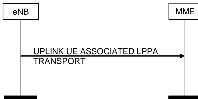
Figure 8.17.2.2-1: UPLINK UE ASSOCIATED LPPA TRANSPORT Procedure
