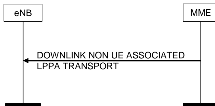
Figure 8.17.2.3-1: DOWNLINK NON UE ASSOCIATED LPPA Transport Procedure
