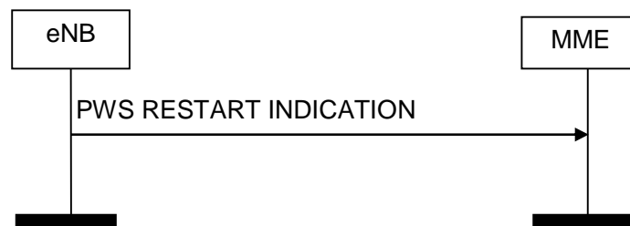
Figure 8.12.3.2-1: PWS Restart Indication procedure. Successful operation.
