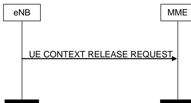
Figure 8.3.2.2-1: UE Context Release Request procedure. Successful operation.
