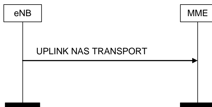
Figure 8.6.2.3-1: UPLINK NAS TRANSPORT Procedure
