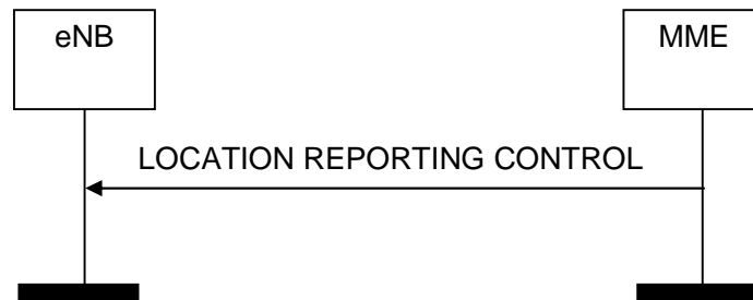
Figure 8.11.1.2-1: Location Reporting Control procedure. Successful operation.
