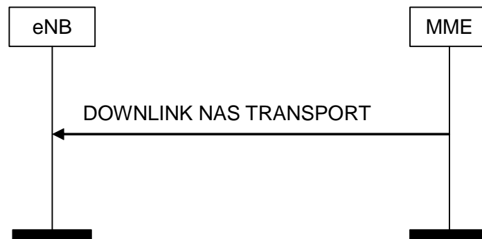
Figure 8.6.2.2-1: DOWNLINK NAS Transport Procedure
