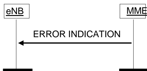
Figure 8.7.2.2-1: Error Indication procedure, MME originated. Successful operation.
