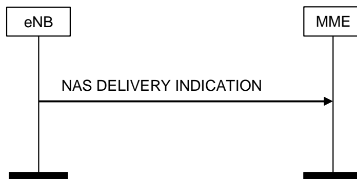
Figure 8.6.2.4a-1: NAS DELIVERY INDICATION Procedure
