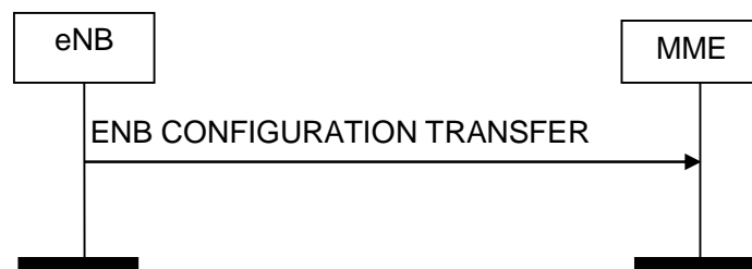
Figure 8.15.2.1-1: eNB Configuration Transfer procedure. Successful operation.
