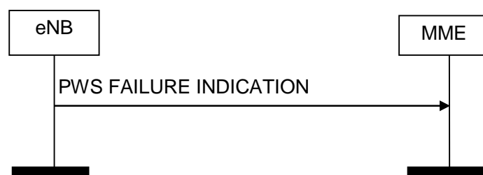
Figure 8.12.4.2-1: PWS Failure Indication procedure. Successful operation.
