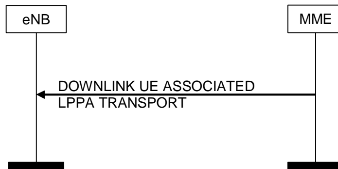
Figure 8.17.2.1-1: DOWNLINK UE ASSOCIATED LPPA Transport Procedure
