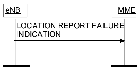
Figure 8.11.2.2-1: Location Report Failure Indication procedure.
