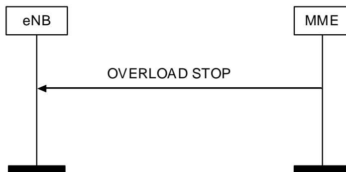
Figure 8.7.7.2.-1: Overload Stop procedure
