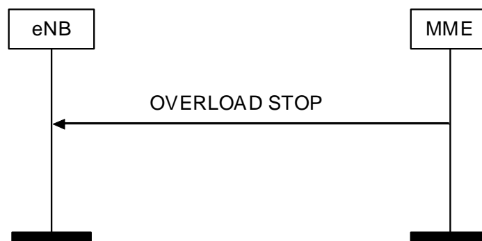
Figure 8.7.7.2.-1: Overload Stop procedure
