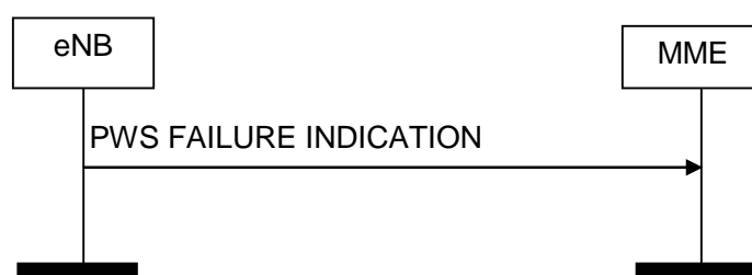
Figure 8.12.4.2-1: PWS Failure Indication procedure. Successful operation.
