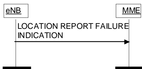
Figure 8.11.2.2-1: Location Report Failure Indication procedure.
