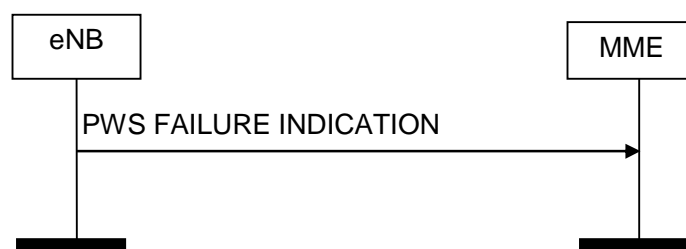
Figure 8.12.4.2-1: PWS Failure Indication procedure. Successful operation.
