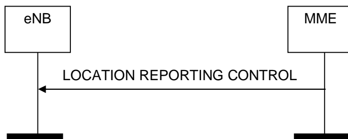
Figure 8.11.1.2-1: Location Reporting Control procedure. Successful operation.
