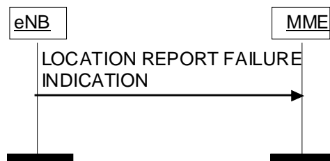
Figure 8.11.2.2-1: Location Report Failure Indication procedure.
