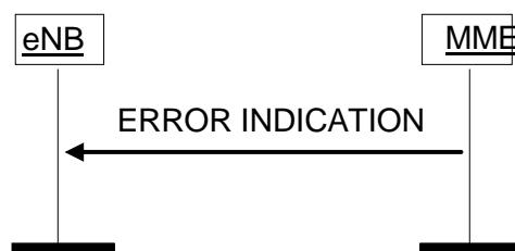
Figure 8.7.2.2-1: Error Indication procedure, MME originated. Successful operation.
