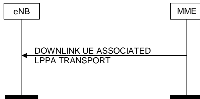
Figure 8.17.2.1-1: DOWNLINK UE ASSOCIATED LPPA Transport Procedure
