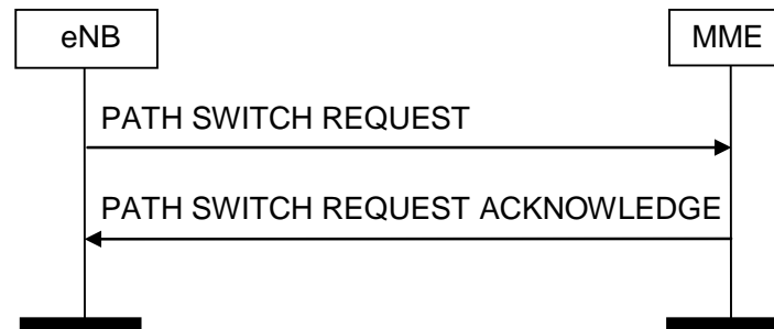
Figure 8.4.4.2-1: Path switch request: successful operation
