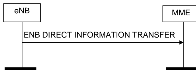
Figure 8.13.1.2-1: ENB Direct Information Transfer procedure. Successful operation.
