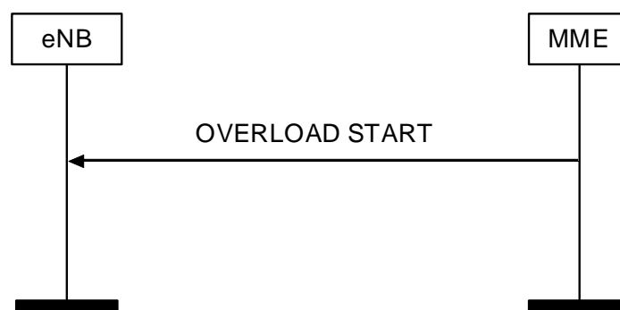
Figure 8.7.6.2-1: Overload Start procedure
