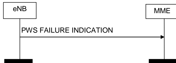
Figure 8.12.4.2-1: PWS Failure Indication procedure. Successful operation.
