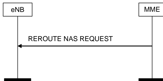
Figure 8.6.2.5-1: Reroute NAS Request Procedure
