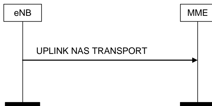
Figure 8.6.2.3-1: UPLINK NAS TRANSPORT Procedure
