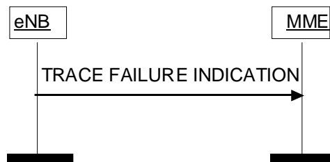
Figure 8.10.2.2-1: Trace Failure Indication procedure.
