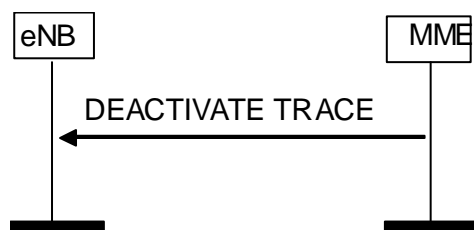
Figure 8.10.3.2-1: Deactivate Trace procedure. Successful operation.
