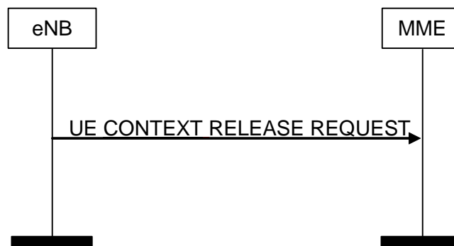
Figure 8.3.2.2-1: UE Context Release Request procedure. Successful operation.
