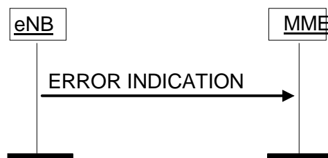
Figure 8.7.2.2-2: Error Indication procedure, eNB originated. Successful operation.
