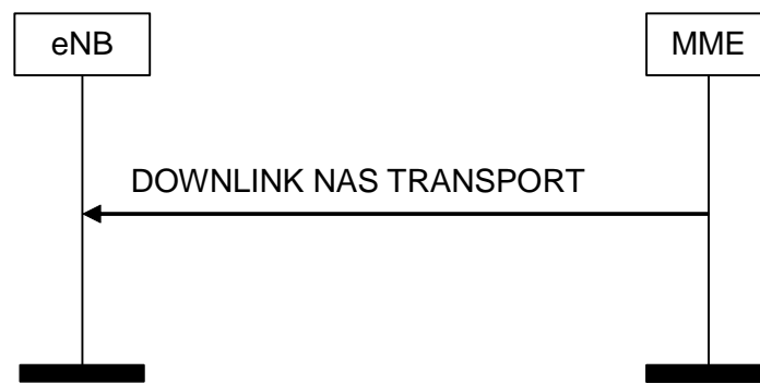
Figure 8.6.2.2-1: DOWNLINK NAS Transport Procedure
