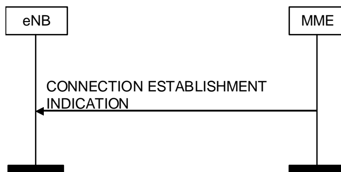
Figure 8.3.9.2-1: Connection Establishment Indication procedure. Successful operation.
