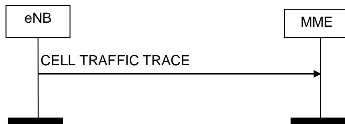
Figure 8.10.4.2-1: Cell Traffic Trace procedure. Successful operation.
