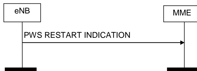
Figure 8.12.3.2-1: PWS Restart Indication procedure. Successful operation.
