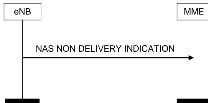
Figure 8.6.2.4-1: NAS NON DELIVERY INDICATION Procedure
