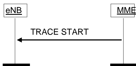
Figure 8.10.1.2-1: Trace Start procedure.
