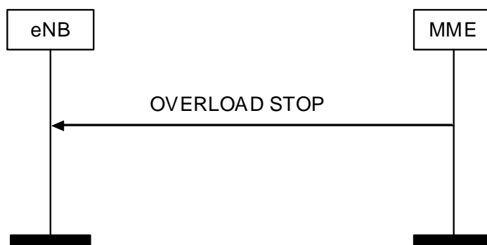
Figure 8.7.7.2.-1: Overload Stop procedure
