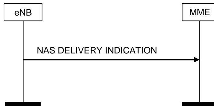
Figure 8.6.2.4a-1: NAS DELIVERY INDICATION Procedure
