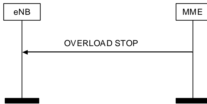
Figure 8.7.7.2.-1: Overload Stop procedure
