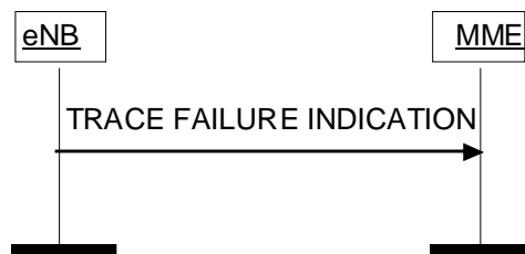
Figure 8.10.2.2-1: Trace Failure Indication procedure.
