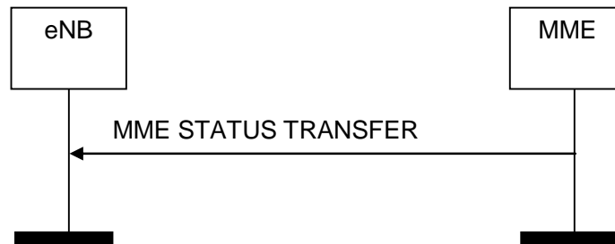
Figure 8.4.7.2-1: MME Status Transfer procedure
