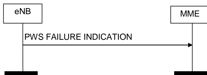
Figure 8.12.4.2-1: PWS Failure Indication procedure. Successful operation.
