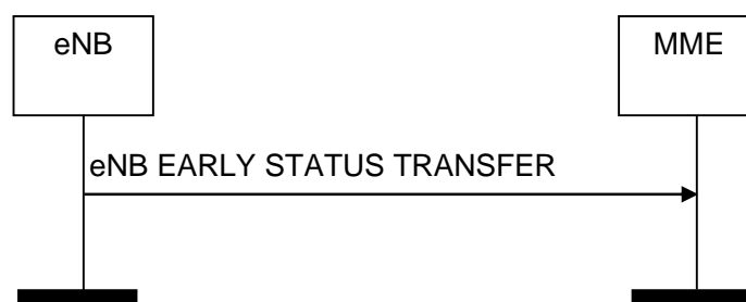
Figure 8.4.9.2-1: eNB Early Status Transfer procedure
