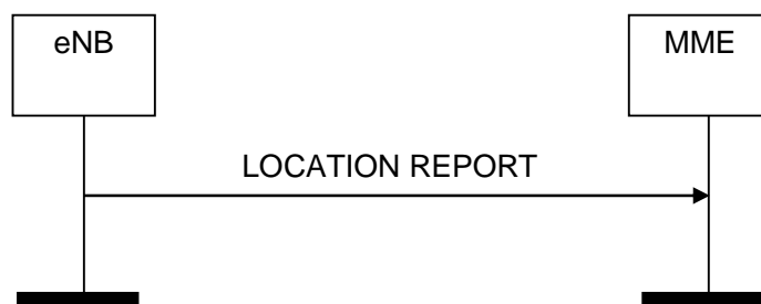
Figure 8.11.3.2-1: Location Report procedure. Successful operation.
