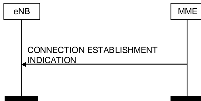
Figure 8.3.9.2-1: Connection Establishment Indication procedure. Successful operation.
