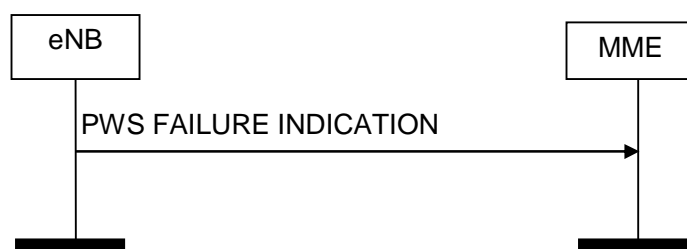
Figure 8.12.4.2-1: PWS Failure Indication procedure. Successful operation.
