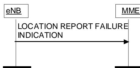
Figure 8.11.2.2-1: Location Report Failure Indication procedure.
