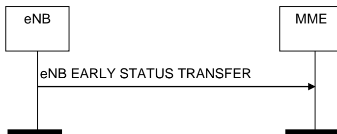
Figure 8.4.9.2-1: eNB Early Status Transfer procedure
