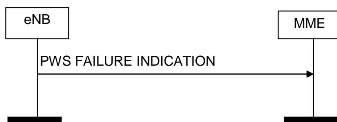
Figure 8.12.4.2-1: PWS Failure Indication procedure. Successful operation.
