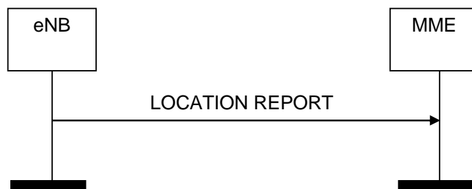
Figure 8.11.3.2-1: Location Report procedure. Successful operation.
