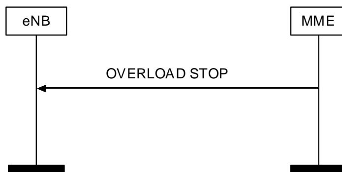
Figure 8.7.7.2.-1: Overload Stop procedure
