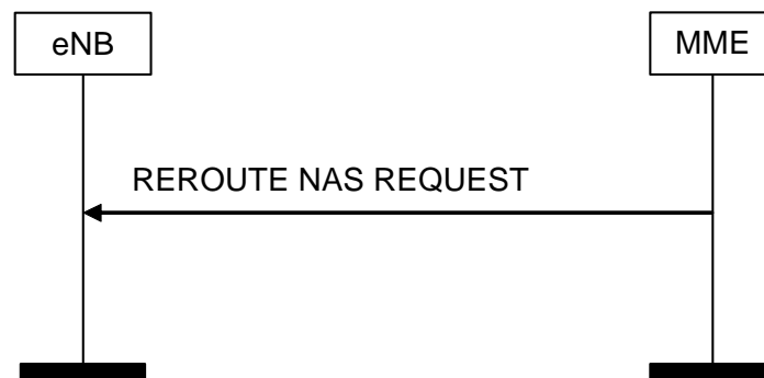
Figure 8.6.2.5-1: Reroute NAS Request Procedure
