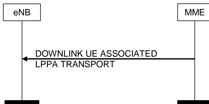
Figure 8.17.2.1-1: DOWNLINK UE ASSOCIATED LPPA Transport Procedure
