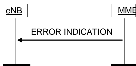
Figure 8.7.2.2-1: Error Indication procedure, MME originated. Successful operation.
