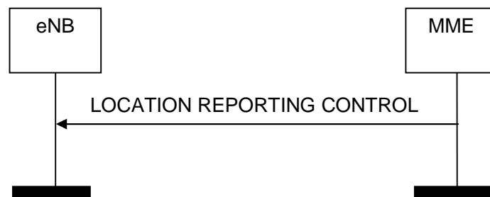
Figure 8.11.1.2-1: Location Reporting Control procedure. Successful operation.
