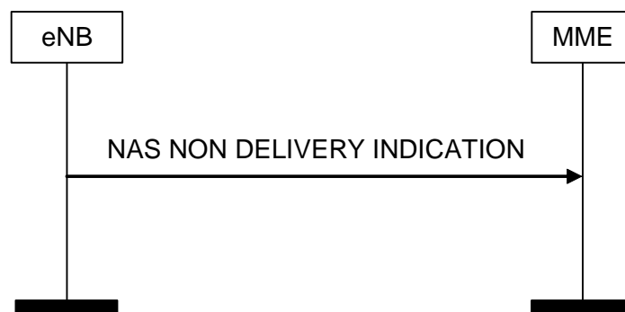
Figure 8.6.2.4-1: NAS NON DELIVERY INDICATION Procedure
