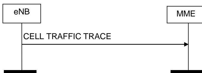
Figure 8.10.4.2-1: Cell Traffic Trace procedure. Successful operation.
