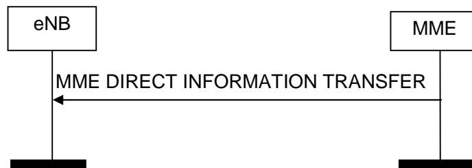
Figure 8.14.1.2-1: MME Direct Information Transfer procedure. Successful operation.
