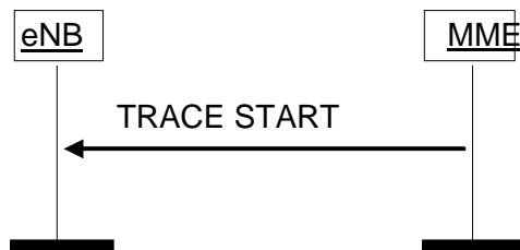
Figure 8.10.1.2-1: Trace Start procedure.
