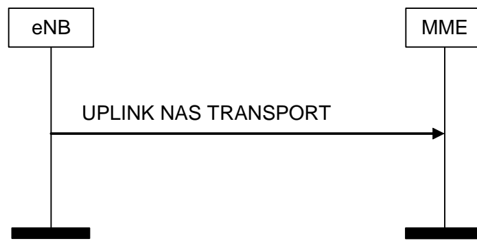
Figure 8.6.2.3-1: UPLINK NAS TRANSPORT Procedure
