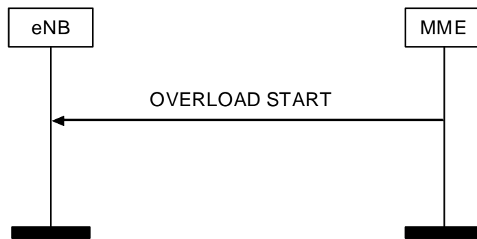
Figure 8.7.6.2-1: Overload Start procedure
