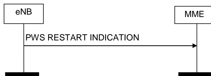
Figure 8.12.3.2-1: PWS Restart Indication procedure. Successful operation.
