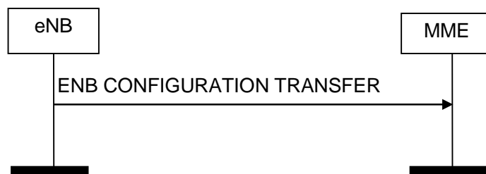
Figure 8.15.2.1-1: eNB Configuration Transfer procedure. Successful operation.
