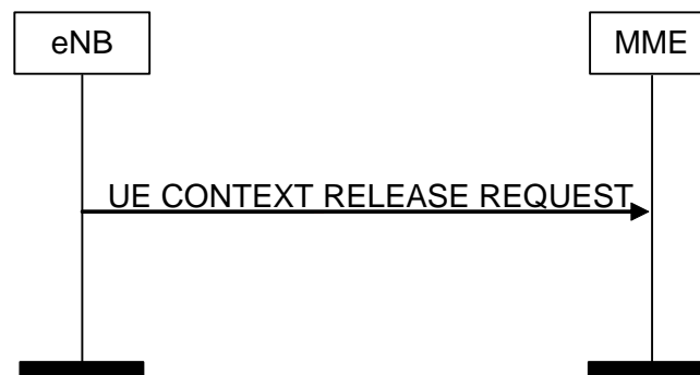
Figure 8.3.2.2-1: UE Context Release Request procedure. Successful operation.
