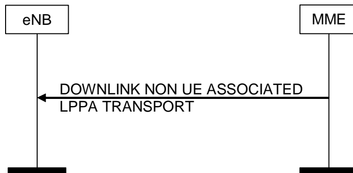
Figure 8.17.2.3-1: DOWNLINK NON UE ASSOCIATED LPPA Transport Procedure
