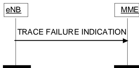
Figure 8.10.2.2-1: Trace Failure Indication procedure.
