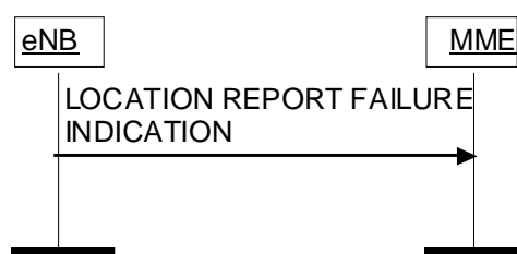
Figure 8.11.2.2-1: Location Report Failure Indication procedure.
