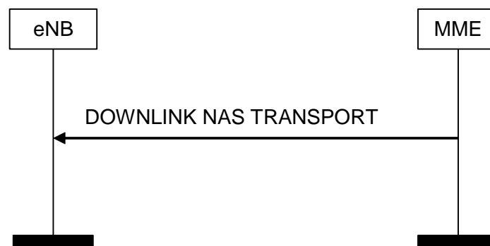
Figure 8.6.2.2-1: DOWNLINK NAS Transport Procedure
