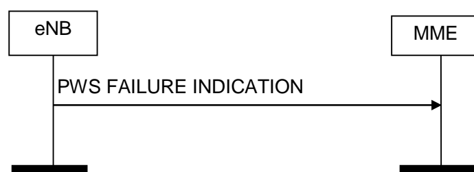
Figure 8.12.4.2-1: PWS Failure Indication procedure. Successful operation.
