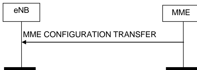
Figure 8.16.2.1-1: MME Configuration Transfer procedure. Successful operation.
