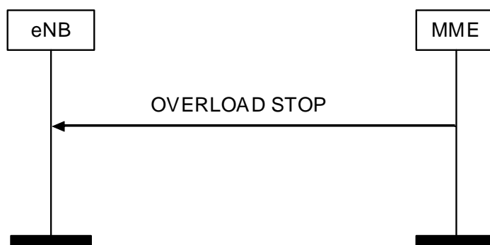
Figure 8.7.7.2.-1: Overload Stop procedure
