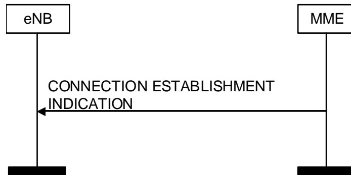
Figure 8.3.9.2-1: Connection Establishment Indication procedure. Successful operation.
