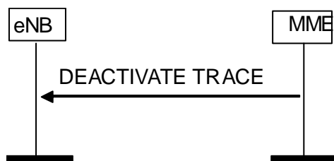
Figure 8.10.3.2-1: Deactivate Trace procedure. Successful operation.
