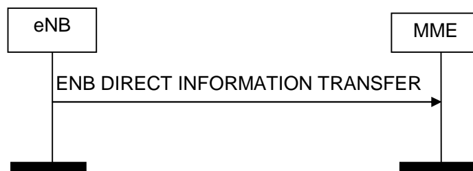
Figure 8.13.1.2-1: ENB Direct Information Transfer procedure. Successful operation.
