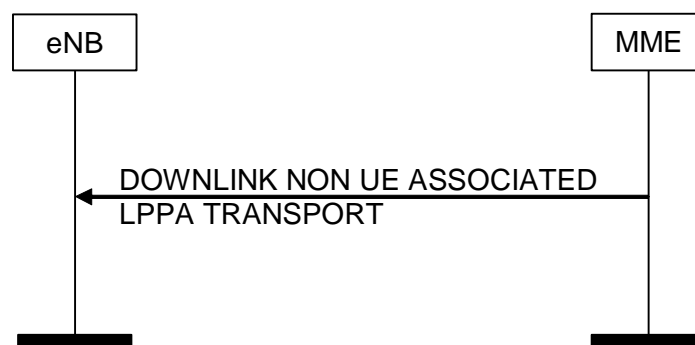
Figure 8.17.2.3-1: DOWNLINK NON UE ASSOCIATED LPPA Transport Procedure
