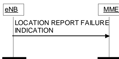
Figure 8.11.2.2-1: Location Report Failure Indication procedure.
