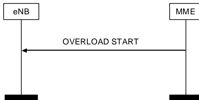
Figure 8.7.6.2-1: Overload Start procedure
