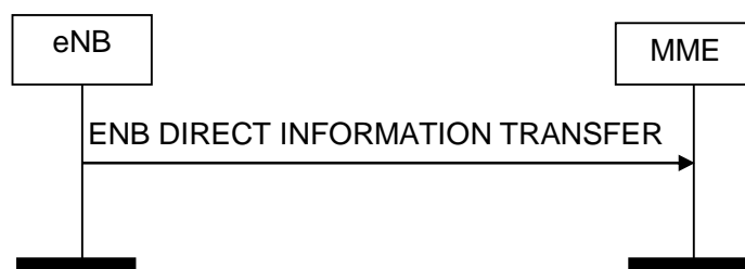
Figure 8.13.1.2-1: ENB Direct Information Transfer procedure. Successful operation.
