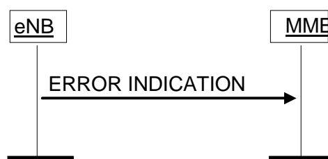
Figure 8.7.2.2-2: Error Indication procedure, eNB originated. Successful operation.
