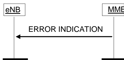
Figure 8.7.2.2-1: Error Indication procedure, MME originated. Successful operation.
