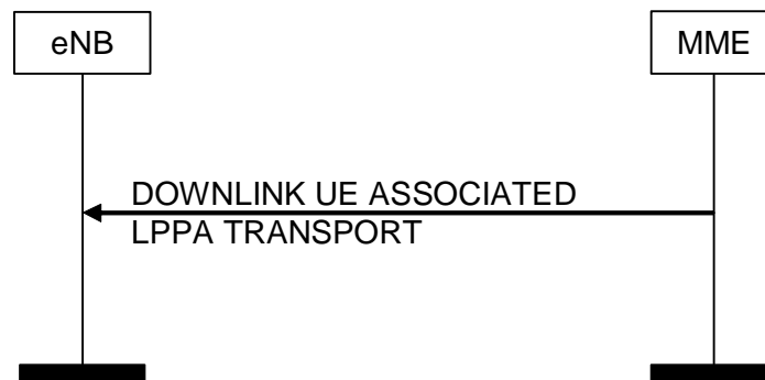
Figure 8.17.2.1-1: DOWNLINK UE ASSOCIATED LPPA Transport Procedure
