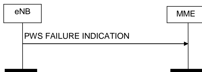
Figure 8.12.4.2-1: PWS Failure Indication procedure. Successful operation.
