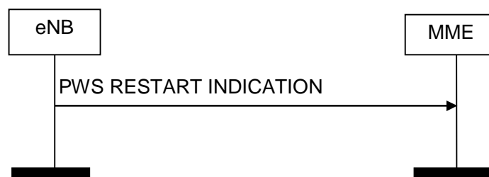
Figure 8.12.3.2-1: PWS Restart Indication procedure. Successful operation.
