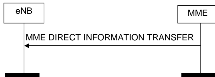
Figure 8.14.1.2-1: MME Direct Information Transfer procedure. Successful operation.
