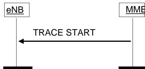
Figure 8.10.1.2-1: Trace Start procedure.
