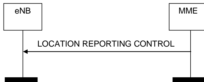
Figure 8.11.1.2-1: Location Reporting Control procedure. Successful operation.
