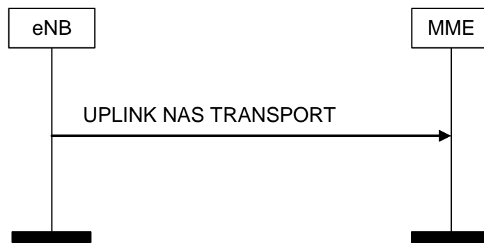
Figure 8.6.2.3-1: UPLINK NAS TRANSPORT Procedure
