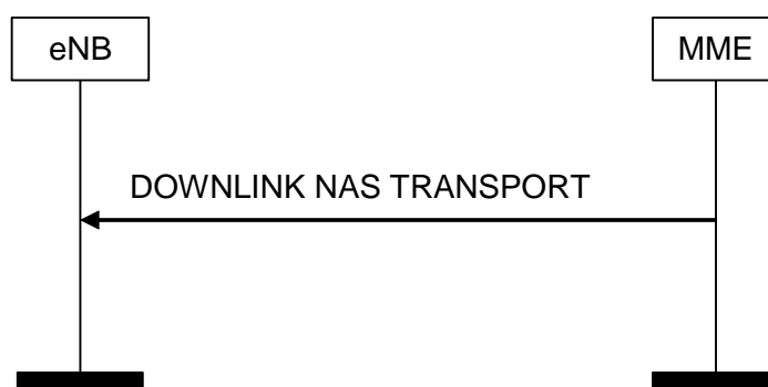
Figure 8.6.2.2-1: DOWNLINK NAS Transport Procedure
