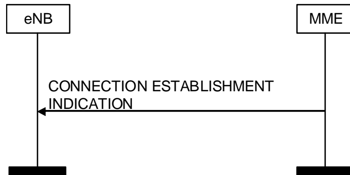
Figure 8.3.9.2-1: Connection Establishment Indication procedure. Successful operation.
