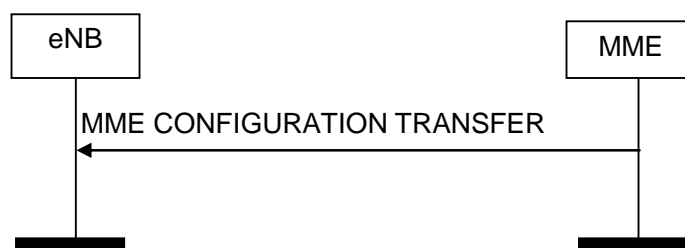
Figure 8.16.2.1-1: MME Configuration Transfer procedure. Successful operation.
