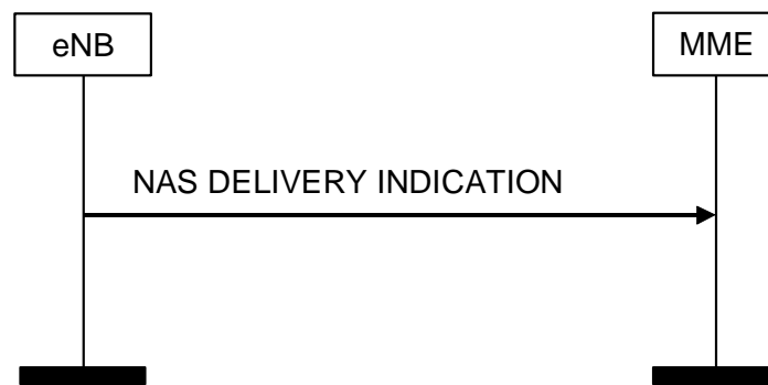
Figure 8.6.2.4a-1: NAS DELIVERY INDICATION Procedure
