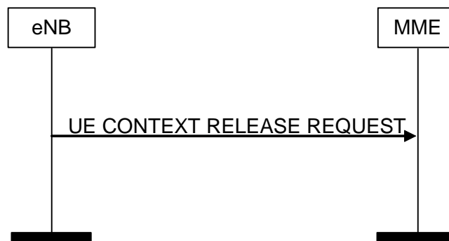
Figure 8.3.2.2-1: UE Context Release Request procedure. Successful operation.
