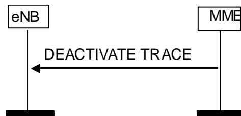
Figure 8.10.3.2-1: Deactivate Trace procedure. Successful operation.
