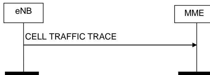
Figure 8.10.4.2-1: Cell Traffic Trace procedure. Successful operation.
