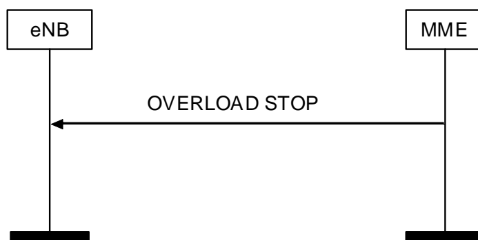
Figure 8.7.7.2.-1: Overload Stop procedure
