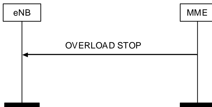
Figure 8.7.7.2.-1: Overload Stop procedure
