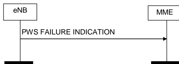
Figure 8.12.4.2-1: PWS Failure Indication procedure. Successful operation.
