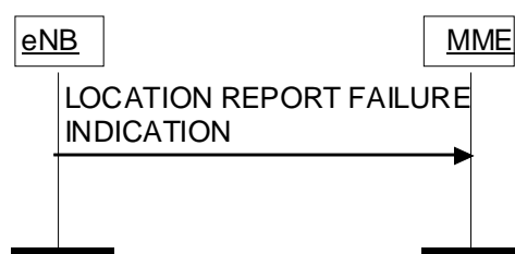
Figure 8.11.2.2-1: Location Report Failure Indication procedure.
