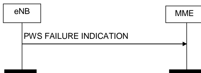
Figure 8.12.4.2-1: PWS Failure Indication procedure. Successful operation.
