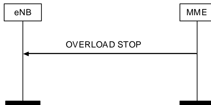
Figure 8.7.7.2.-1: Overload Stop procedure
