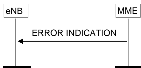
Figure 8.7.2.2-1: Error Indication procedure, MME originated. Successful operation.
