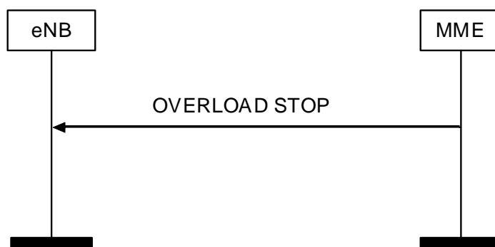
Figure 8.7.7.2.-1: Overload Stop procedure
