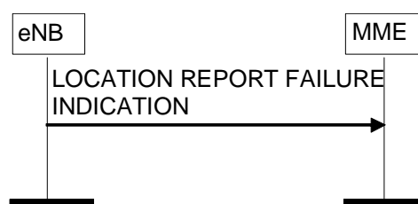
Figure 8.11.2.2-1: Location Report Failure Indication procedure.
