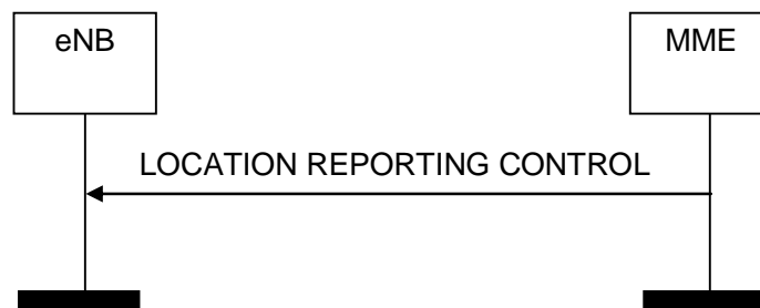
Figure 8.11.1.2-1: Location Reporting Control procedure. Successful operation.
