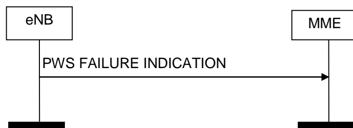
Figure 8.12.4.2-1: PWS Failure Indication procedure. Successful operation.
