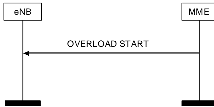
Figure 8.7.6.2-1: Overload Start procedure
