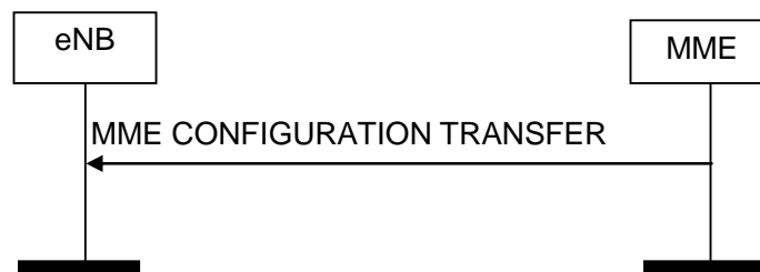
Figure 8.16.2.1-1: MME Configuration Transfer procedure. Successful operation.
