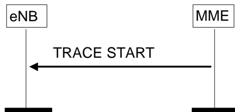
Figure 8.10.1.2-1: Trace Start procedure.
