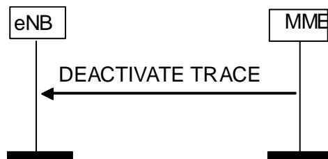
Figure 8.10.3.2-1: Deactivate Trace procedure. Successful operation.
