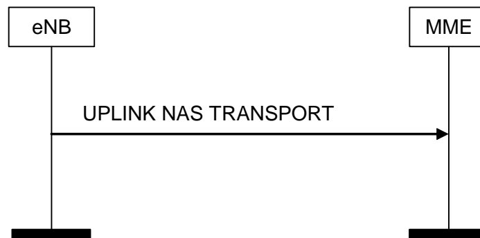
Figure 8.6.2.3-1: UPLINK NAS TRANSPORT Procedure
