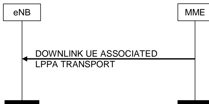
Figure 8.17.2.1-1: DOWNLINK UE ASSOCIATED LPPA Transport Procedure
