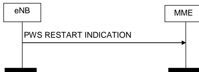
Figure 8.12.3.2-1: PWS Restart Indication procedure. Successful operation.
