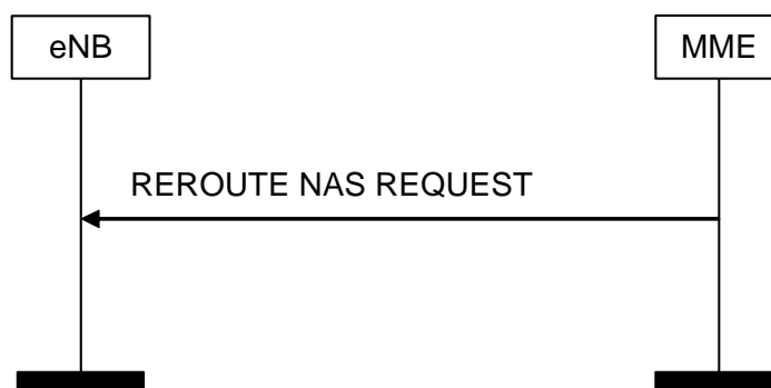
Figure 8.6.2.5-1: Reroute NAS Request Procedure
