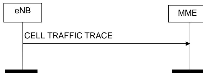
Figure 8.10.4.2-1: Cell Traffic Trace procedure. Successful operation.
