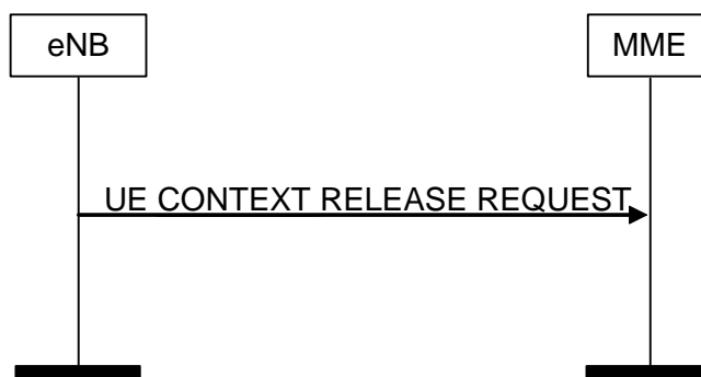
Figure 8.3.2.2-1: UE Context Release Request procedure. Successful operation.
