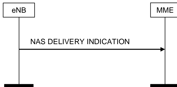
Figure 8.6.2.4a-1: NAS DELIVERY INDICATION Procedure
