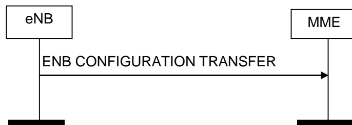
Figure 8.15.2.1-1: eNB Configuration Transfer procedure. Successful operation.
