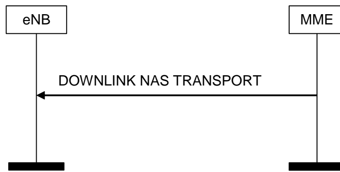
Figure 8.6.2.2-1: DOWNLINK NAS Transport Procedure
