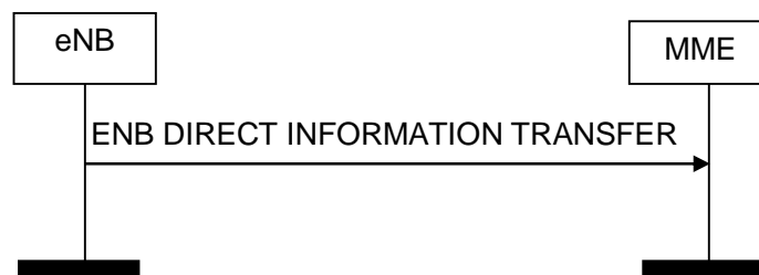
Figure 8.13.1.2-1: ENB Direct Information Transfer procedure. Successful operation.
