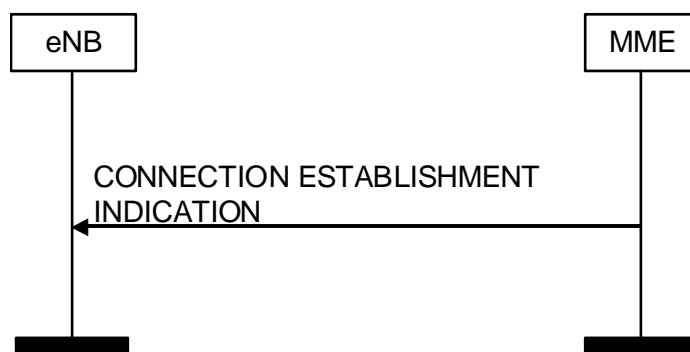
Figure 8.3.9.2-1: Connection Establishment Indication procedure. Successful operation.
