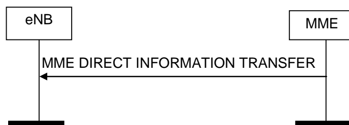
Figure 8.14.1.2-1: MME Direct Information Transfer procedure. Successful operation.
