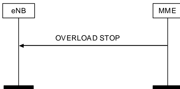
Figure 8.7.7.2.-1: Overload Stop procedure
