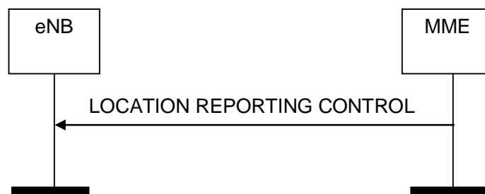
Figure 8.11.1.2-1: Location Reporting Control procedure. Successful operation.
