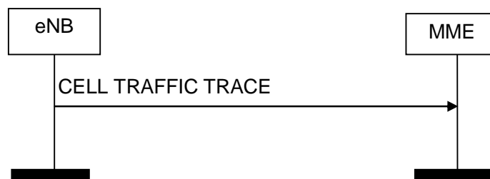
Figure 8.10.4.2-1: Cell Traffic Trace procedure. Successful operation.
