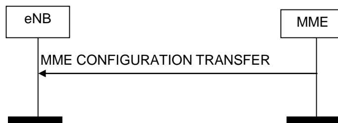
Figure 8.16.2.1-1: MME Configuration Transfer procedure. Successful operation.
