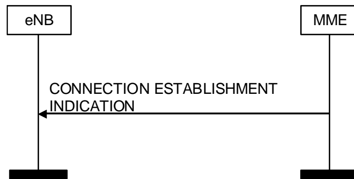
Figure 8.3.9.2-1: Connection Establishment Indication procedure. Successful operation.
