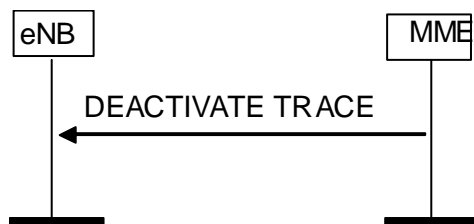
Figure 8.10.3.2-1: Deactivate Trace procedure. Successful operation.
