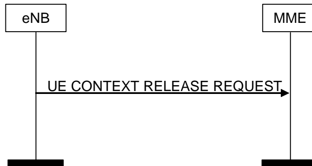
Figure 8.3.2.2-1: UE Context Release Request procedure. Successful operation.
