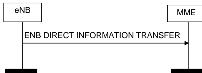
Figure 8.13.1.2-1: ENB Direct Information Transfer procedure. Successful operation.
