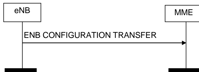
Figure 8.15.2.1-1: eNB Configuration Transfer procedure. Successful operation.
