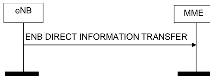
Figure 8.13.1.2-1: ENB Direct Information Transfer procedure. Successful operation.
