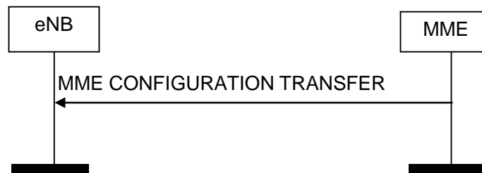
Figure 8.16.2.1-1: MME Configuration Transfer procedure. Successful operation.
