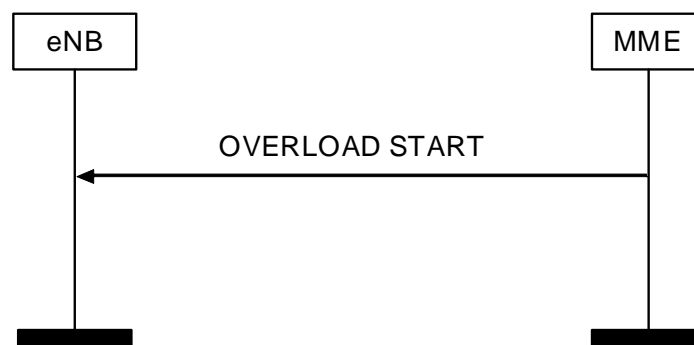
Figure 8.7.6.2-1: Overload Start procedure
