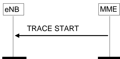
Figure 8.10.1.2-1: Trace Start procedure.
