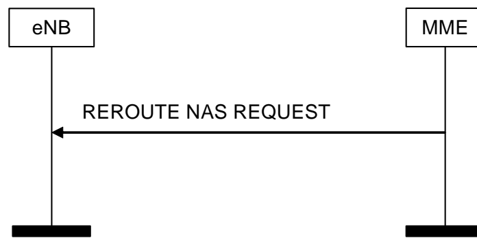
Figure 8.6.2.5-1: Reroute NAS Request Procedure
