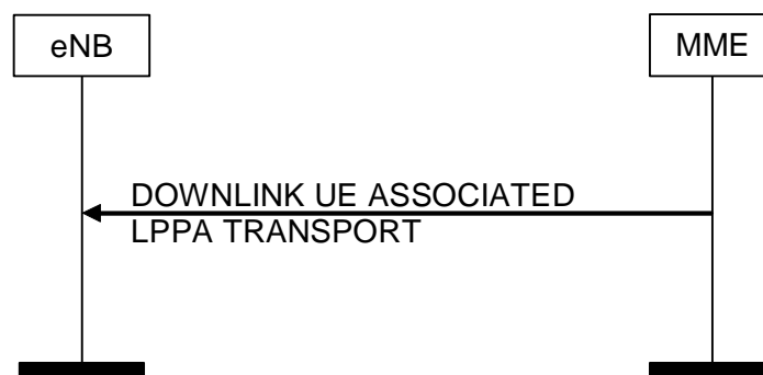
Figure 8.17.2.1-1: DOWNLINK UE ASSOCIATED LPPA Transport Procedure
