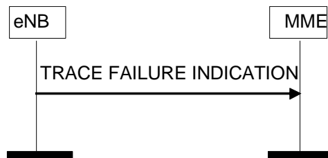
Figure 8.10.2.2-1: Trace Failure Indication procedure.
