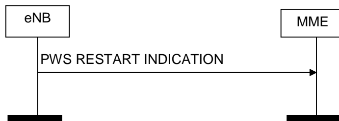
Figure 8.12.3.2-1: PWS Restart Indication procedure. Successful operation.
