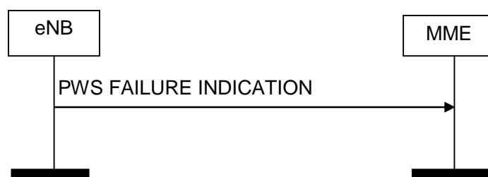
Figure 8.12.4.2-1: PWS Failure Indication procedure. Successful operation.
