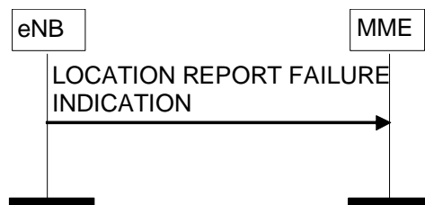
Figure 8.11.2.2-1: Location Report Failure Indication procedure.
