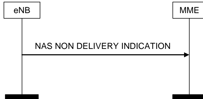
Figure 8.6.2.4-1: NAS NON DELIVERY INDICATION Procedure
