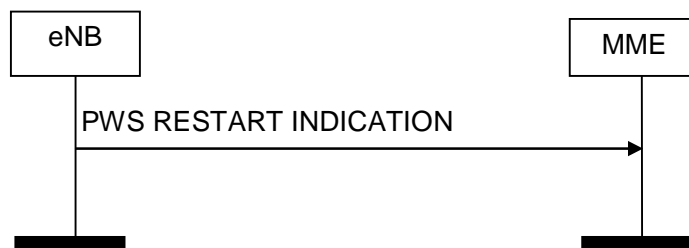
Figure 8.12.3.2-1: PWS Restart Indication procedure. Successful operation.
