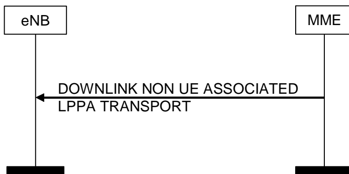
Figure 8.17.2.3-1: DOWNLINK NON UE ASSOCIATED LPPA Transport Procedure
