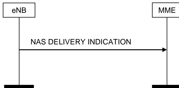
Figure 8.6.2.4a-1: NAS DELIVERY INDICATION Procedure
