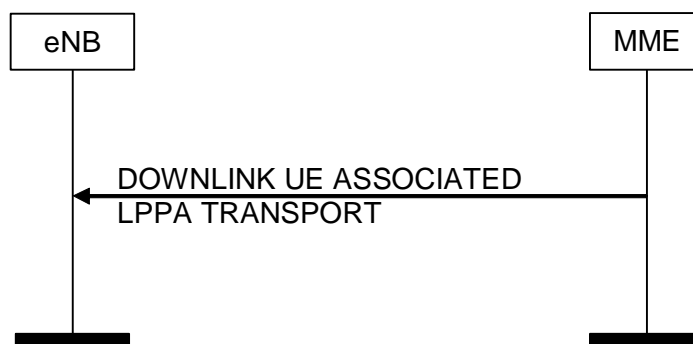
Figure 8.17.2.1-1: DOWNLINK UE ASSOCIATED LPPA Transport Procedure
