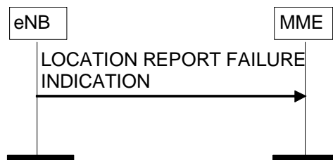
Figure 8.11.2.2-1: Location Report Failure Indication procedure.
