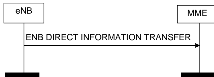
Figure 8.13.1.2-1: ENB Direct Information Transfer procedure. Successful operation.
