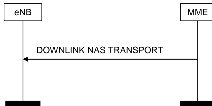
Figure 8.6.2.2-1: DOWNLINK NAS Transport Procedure
