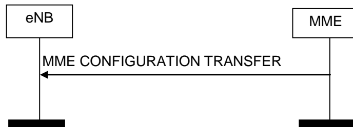
Figure 8.16.2.1-1: MME Configuration Transfer procedure. Successful operation.
