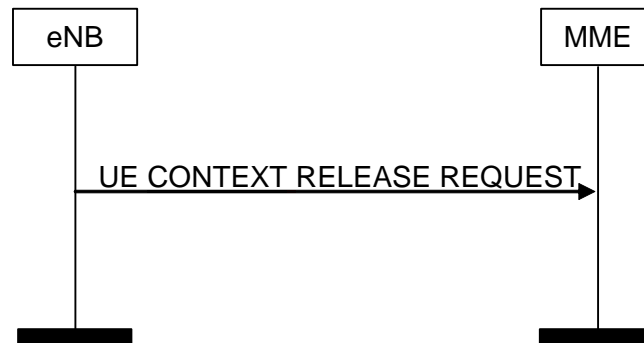
Figure 8.3.2.2-1: UE Context Release Request procedure. Successful operation.
