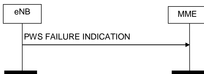
Figure 8.12.4.2-1: PWS Failure Indication procedure. Successful operation.
