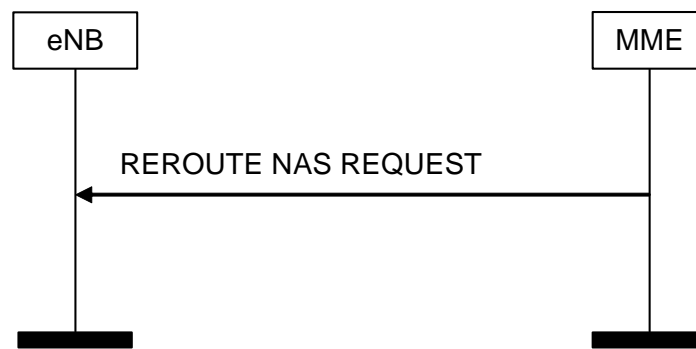
Figure 8.6.2.5-1: Reroute NAS Request Procedure
