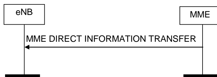
Figure 8.14.1.2-1: MME Direct Information Transfer procedure. Successful operation.
