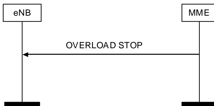
Figure 8.7.7.2.-1: Overload Stop procedure
