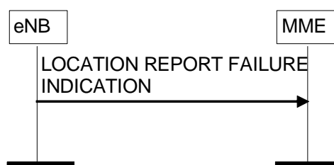
Figure 8.11.2.2-1: Location Report Failure Indication procedure.
