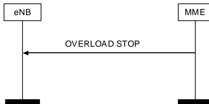
Figure 8.7.7.2.-1: Overload Stop procedure
