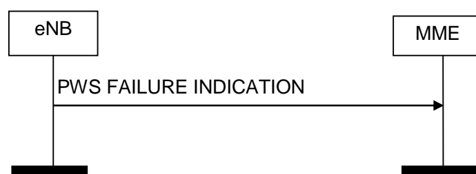
Figure 8.12.4.2-1: PWS Failure Indication procedure. Successful operation.
