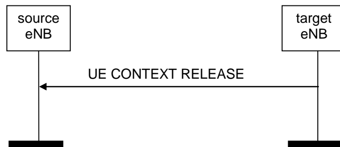
Figure 8.2.3.2-1: UE Context Release, successful operation
