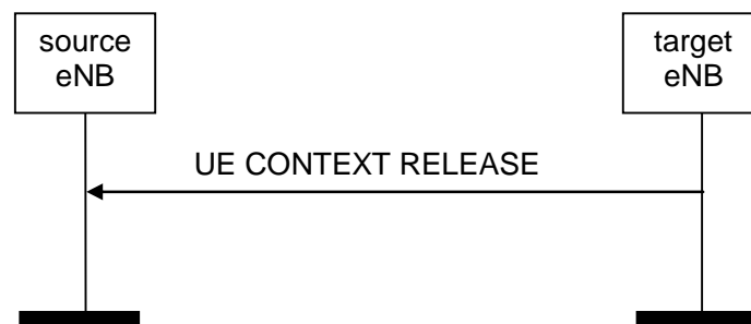
Figure 8.2.3.2-1: UE Context Release, successful operation
