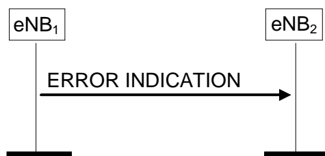
Figure 8.3.2.2-1: Error Indication, successful operation.
