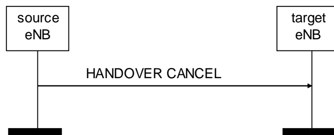
Figure 8.2.4.2-1: Handover Cancel, successful operation
