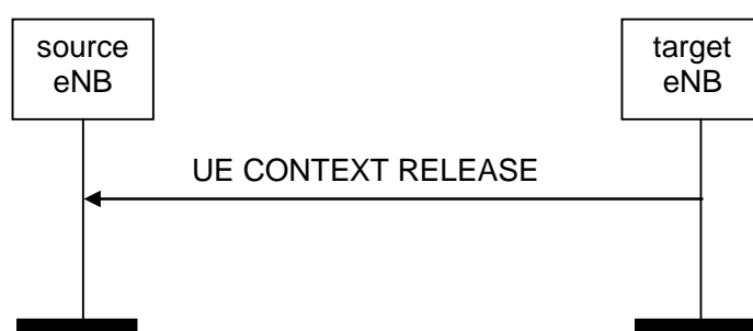
Figure 8.2.3.2-1: UE Context Release, successful operation
