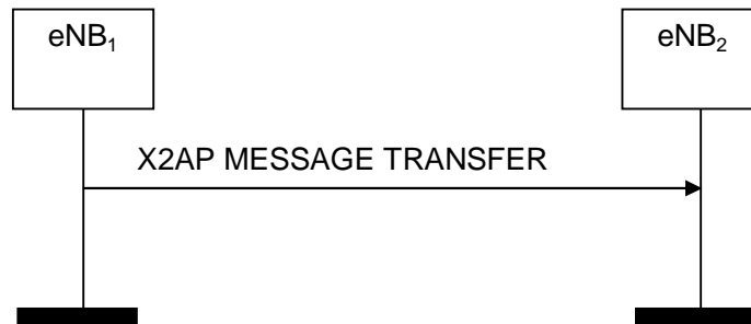
Figure 8.5.2-1: X2AP Message Transfer, successful operation
