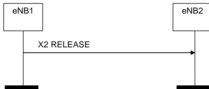
Figure 8.4.2-1: X2AP Release, successful operation
