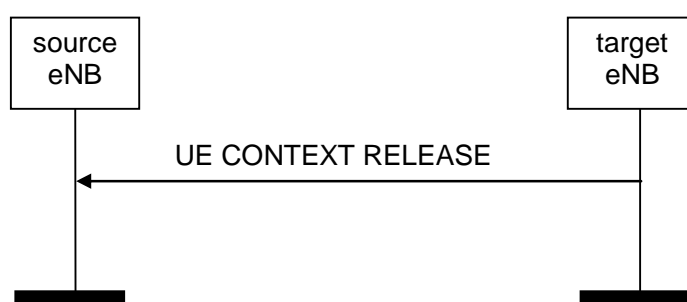
Figure 8.2.3.2-1: UE Context Release, successful operation
