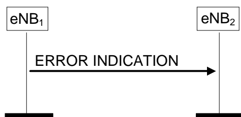
Figure 8.3.2.2-1: Error Indication, successful operation.
