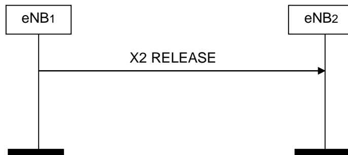
Figure 8.4.2-1: X2AP Release, successful operation
