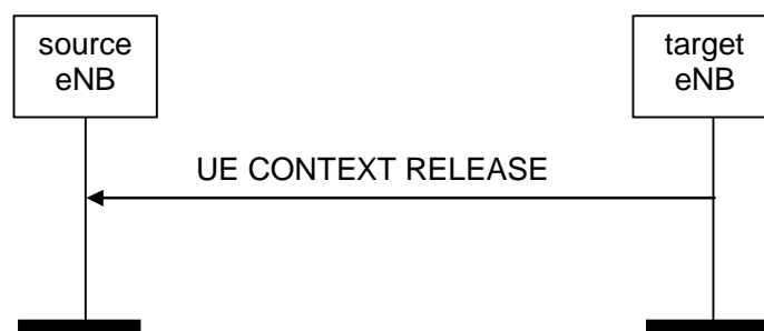
Figure 8.2.3.2-1: UE Context Release, successful operation for handover
