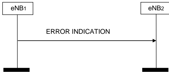
Figure 8.3.2.2-1: Error Indication, successful operation.
