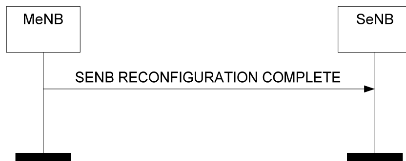
Figure 8.6.2.2-1: SeNB Reconfiguration Complete procedure, successful operation.
