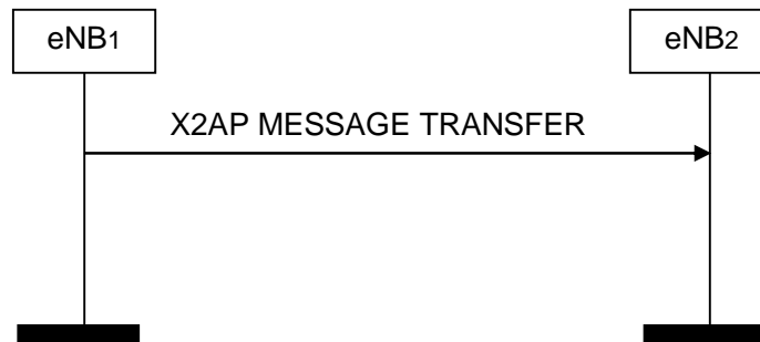
Figure 8.5.2-1: X2AP Message Transfer, successful operation
