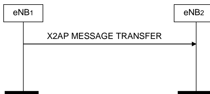
Figure 8.5.2-1: X2AP Message Transfer, successful operation
