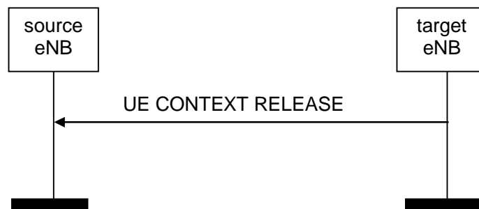
Figure 8.2.3.2-1: UE Context Release, successful operation for handover
