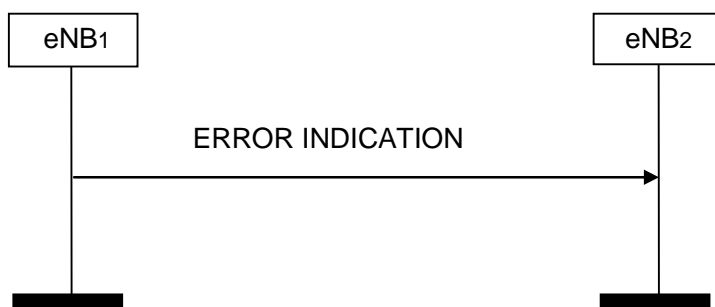
Figure 8.3.2.2-1: Error Indication, successful operation.
