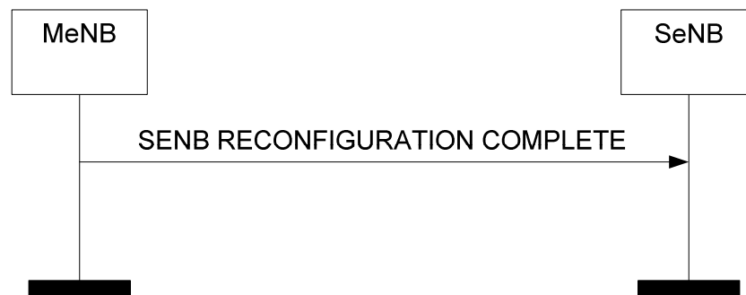
Figure 8.6.2.2-1: SeNB Reconfiguration Complete procedure, successful operation.
