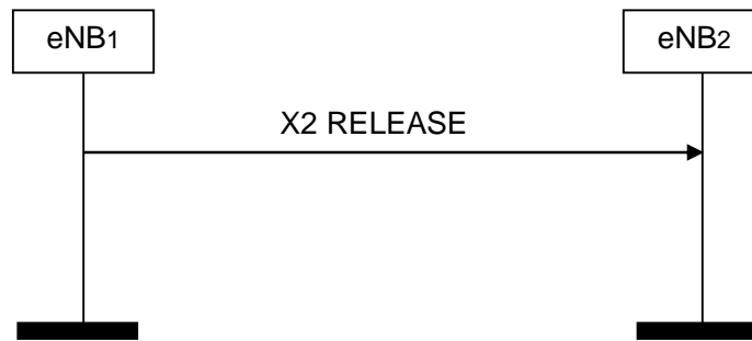
Figure 8.4.2-1: X2AP Release, successful operation
