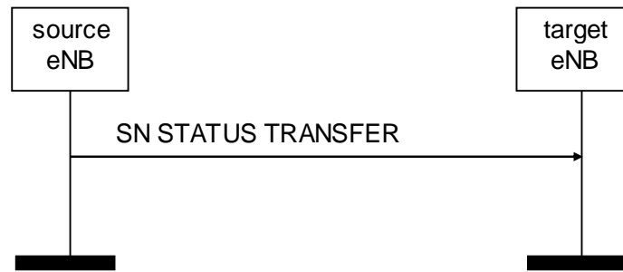
Figure 8.2.2.2-1: SN Status Transfer, successful operation
