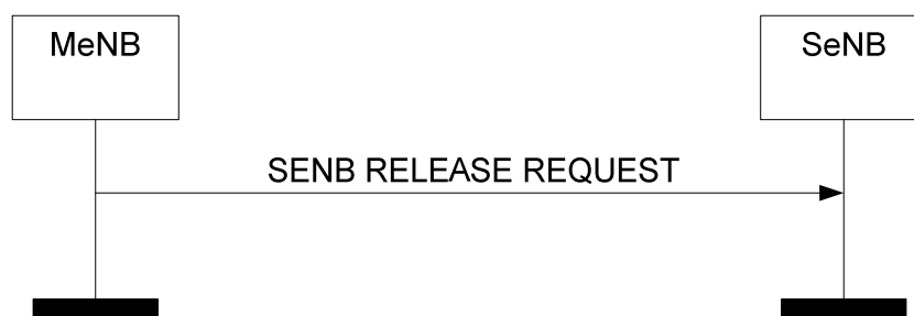
Figure 8.6.5.2-1: MeNB initiated SeNB Release, successful operation
