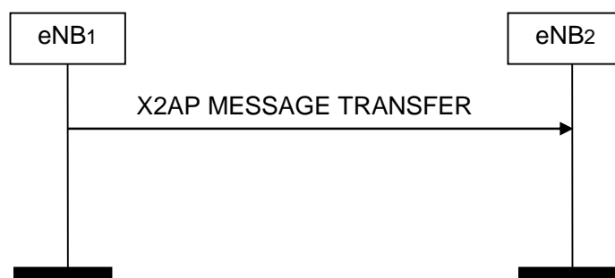
Figure 8.5.2-1: X2AP Message Transfer, successful operation
