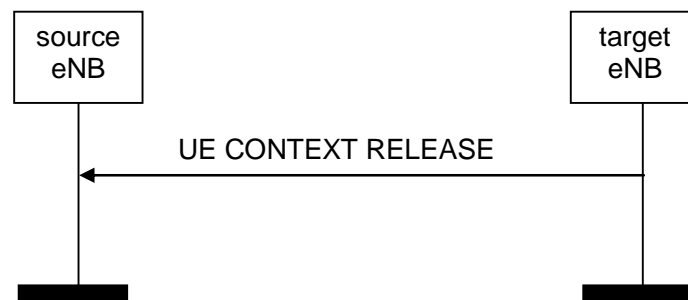
Figure 8.2.3.2-1: UE Context Release, successful operation for handover
