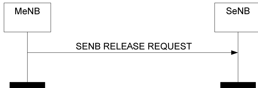
Figure 8.6.5.2-1: MeNB initiated SeNB Release, successful operation
