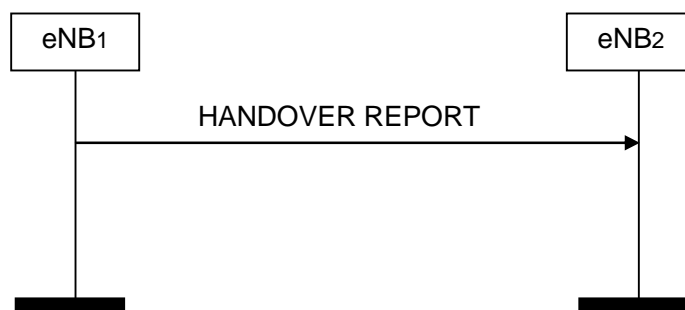
Figure 8.3.10.2-1: Handover Report, successful operation
