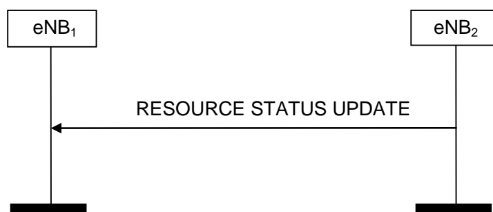
Figure 8.3.7.2-1: Resource Status Reporting, successful operation
