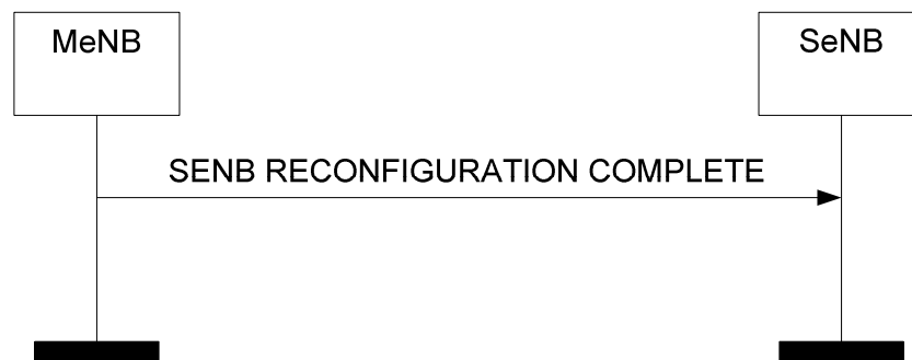
Figure 8.6.2.2-1: SeNB Reconfiguration Complete procedure, successful operation.
