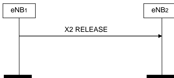
Figure 8.4.2-1: X2AP Release, successful operation
