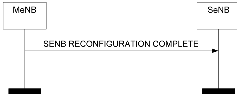
Figure 8.6.2.2-1: SeNB Reconfiguration Complete procedure, successful operation.
