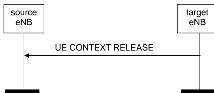
Figure 8.2.3.2-1: UE Context Release, successful operation for handover
