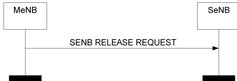
Figure 8.6.5.2-1: MeNB initiated SeNB Release, successful operation
