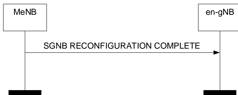
Figure 8.7.5.2-1: SgNB Reconfiguration Complete procedure, successful operation.
