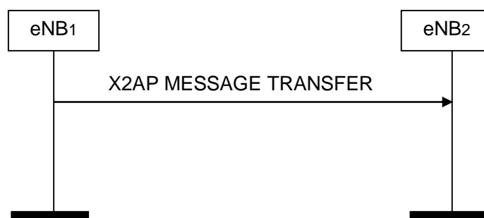
Figure 8.5.2-1: X2AP Message Transfer, successful operation
