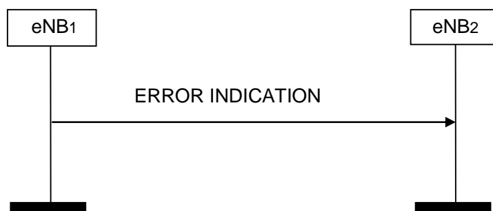
Figure 8.3.2.2-1: Error Indication, successful operation.
