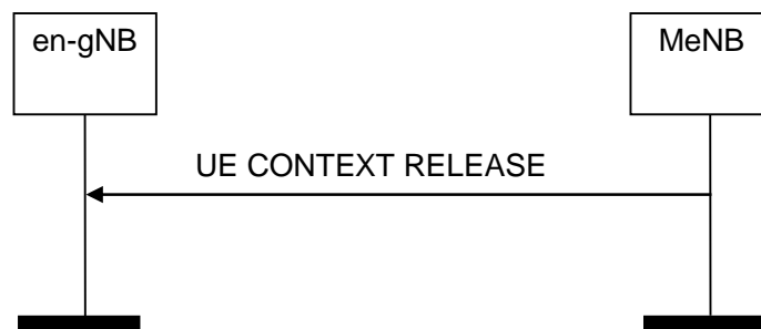
Figure 8.2.3.2-3: UE Context Release, successful operation for EN-DC
