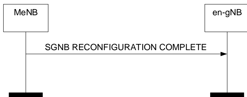
Figure 8.7.5.2-1: SgNB Reconfiguration Complete procedure, successful operation.
