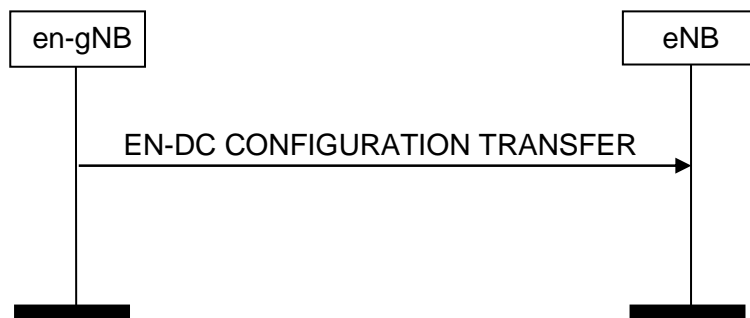
Figure 8.7.18.2-2: en-gNB initiated EN-DC Configuration Transfer, successful operation
