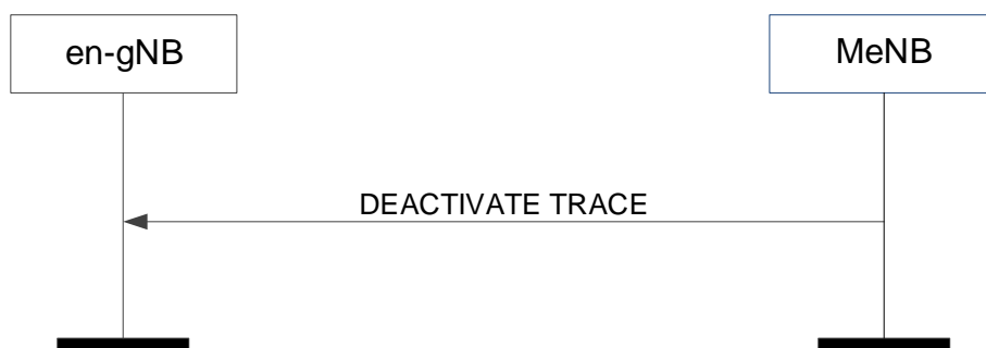
Figure 8.7.20.2-1: Deactivate Trace, successful operation
