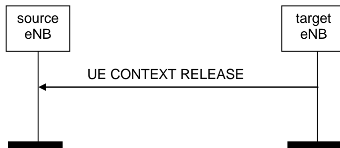
Figure 8.2.3.2-1: UE Context Release, successful operation for handover
