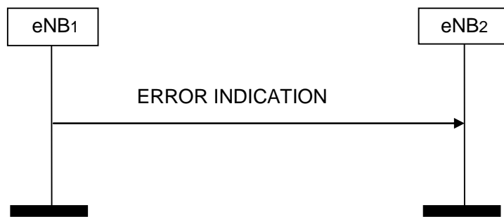
Figure 8.3.2.2-1: Error Indication, successful operation.
