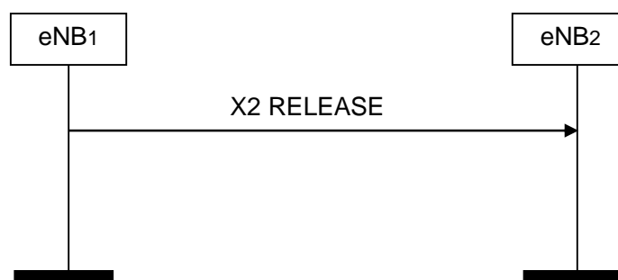
Figure 8.4.2-1: X2AP Release, successful operation
